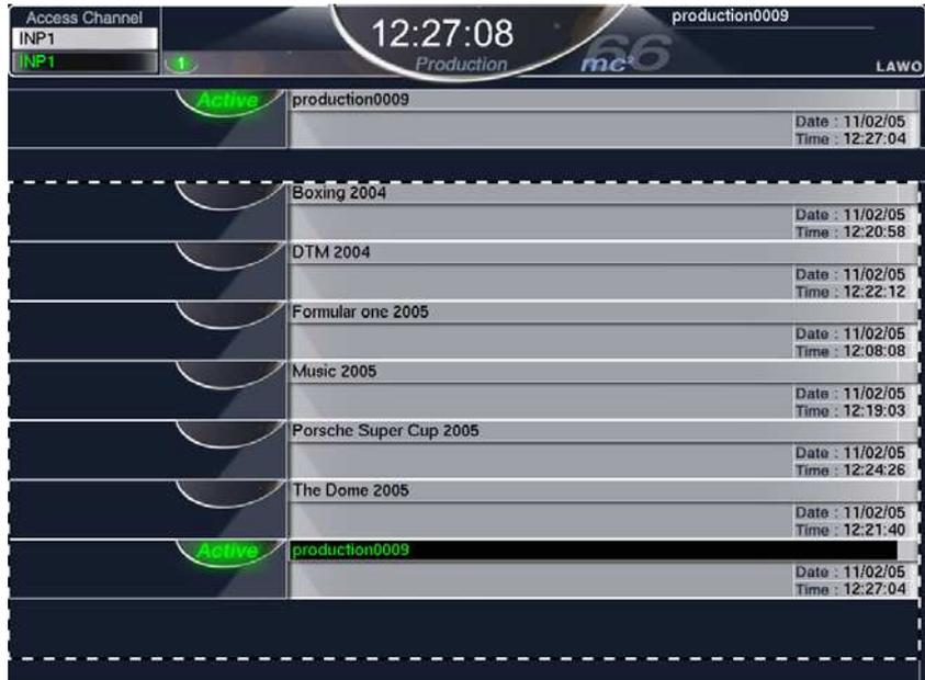
A new entry appears in the productions list with a default name (e.g. **production 0009**). This entry contains all the settings of the console and is time and date stamped. The new production automatically becomes the **Active** production as shown on the display.
