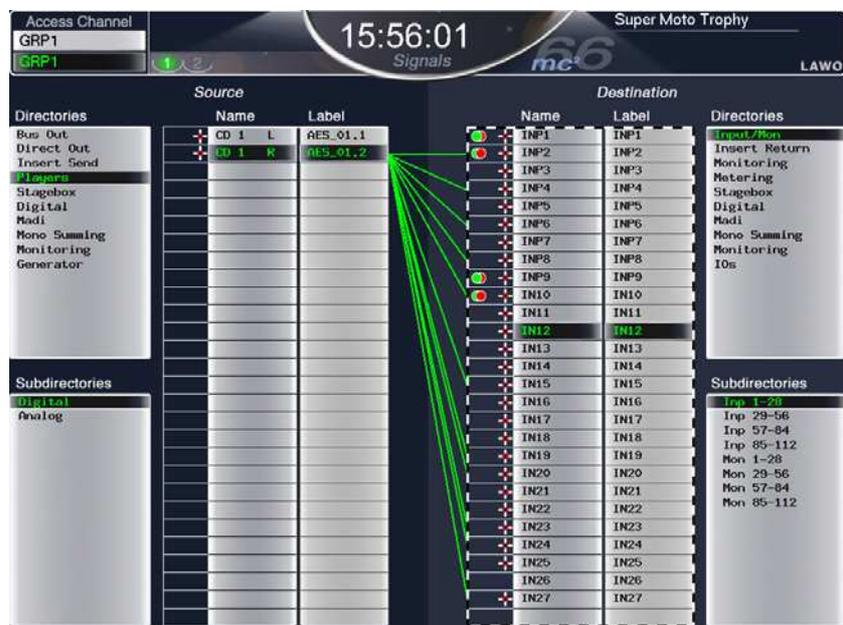
2. Using the trackball or navigation buttons, select the source directory (e.g. **Bus Out**) and sub-directory (e.g. **DOut Sum 1-28**) on the left of the display.
