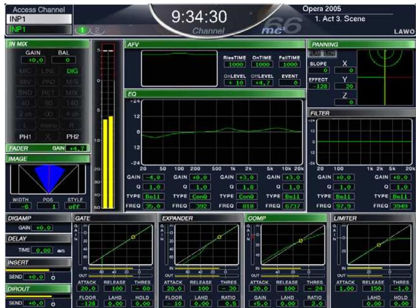
The **Main** display is divided into the same sub sections as the Central Control Section front panel. As you adjust controls, the display updates to reflect your settings.
