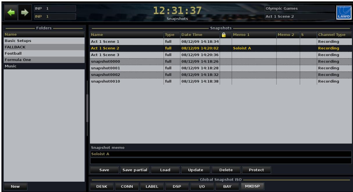
2. Using the trackball or navigation buttons focus on the list of **Folders** on the left hand side of the display.
