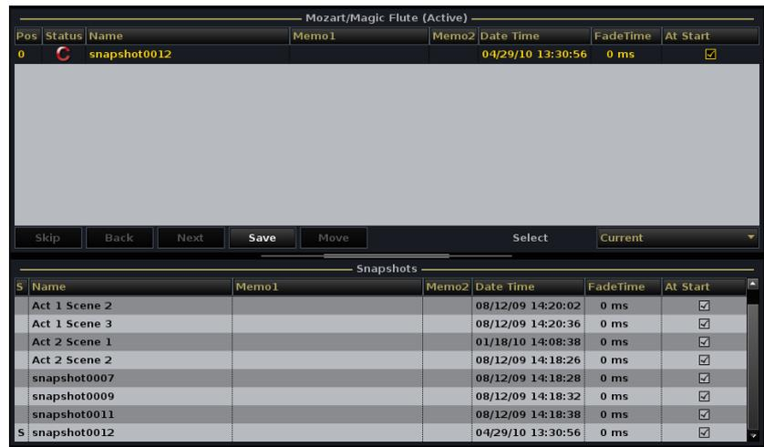
A new snapshot appears below the current selection. If this is the first snapshot to be added to the sequence, then it will appear at the top of the list!
