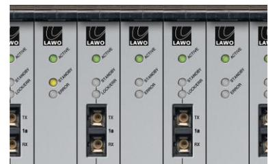
Note that the replaced board now acts as the spare board either until the HD core is restarted or a new DSP configuration is loaded. Following the reconfiguration, boards are utilised from right to left across the HD core, in our example slots 1 to 7 for main DSP resources and slot 8 in standby status.
