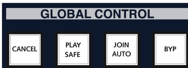
*Once selected, all channels enabled for automation will read data from the Play pass but not write new data.*
