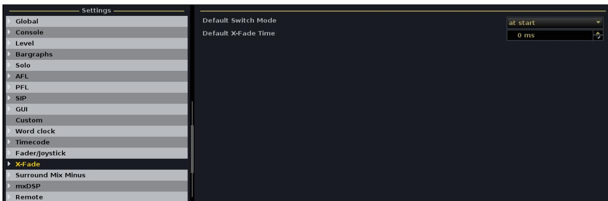
You can set the default switch mode so that switched functions, such as mutes, will change state at the start or end of the cross fade. You can also set the default fade time in 100ms steps.
