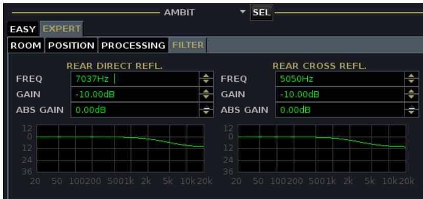
2. Use the REAR DIRECT REFL. and REAR CROSS REFL. parameters to adjust the virtual room reflections applied by the Spatialiser to surround left and right.
