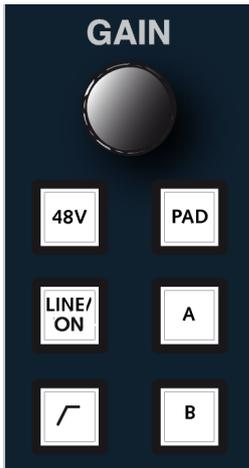
Each microphone pre-amplifier may be remotely controlled in order to set input gain, phantom power, etc. prior to analogue-to-digital conversion. These settings may be controlled either from the fader strip or the Central Control Section. Let's use the dedicated controls on the channel fader strip:
