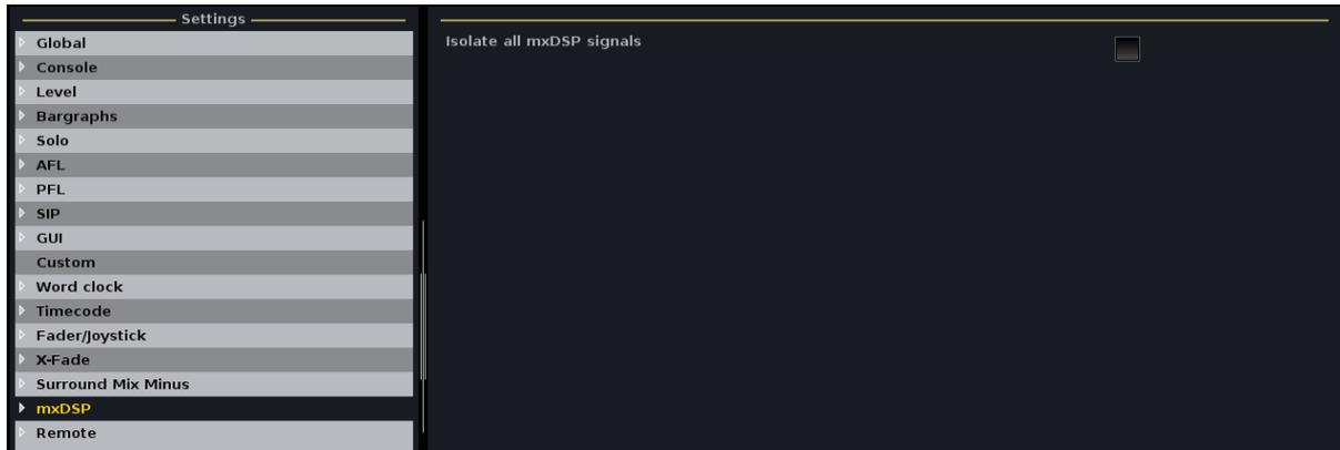
The option determines whether mxDSP signals are affected by snapshot loads:
