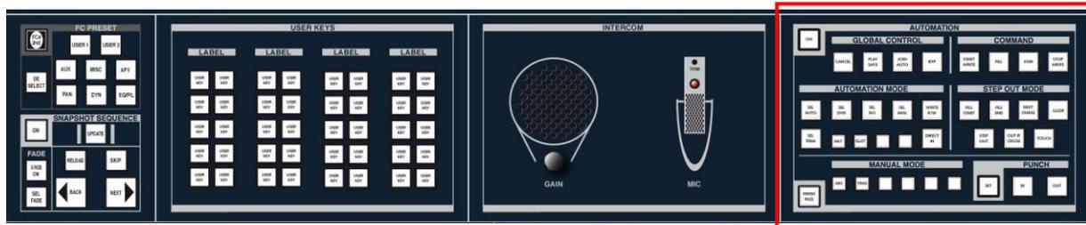
AUTOMATION controls are a standard part of the centre section on the classic mc<sup>2</sup>66.
