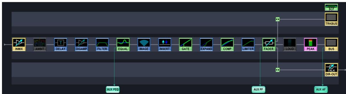
Processing modules such as EQ, Delay, Insert, Comp, etc. can be positioned at any point in the chain, enabling you to change the channel signal flow on a channel-by-channel basis. For example, you could put the Limiter post-fader. Or, the Direct Output pre-delay.
