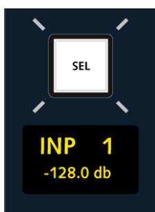
This also provides an overview of source to channel routes without needing to view the **Signal List** display. For example, with **INHERIT SOURCE** selected, if your fader label displays show channel labels then you know there are no sources assigned. Or, if an external controller is making connects within the router, you will be able to see the names of the sources as they are assigned remotely.
