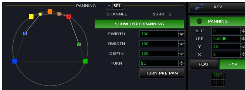
By enabling the **TURN PRE PAN** button (on-screen), you can turn the surround source and then position the rotated source using the joystick.
