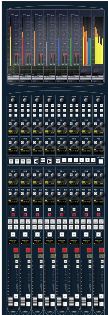
The console's control surface includes both channel and main fader strips. Any fader strip may control any type of channel - input, monitor return, group, sum, auxiliary, VCA or Surround master – allowing you to lay out your source channels and output masters where you want them.
