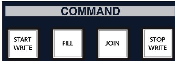
All parameters and modules which have been selected for automation step into write. The **R/W** buttons beside each fader will turn red when in write.
