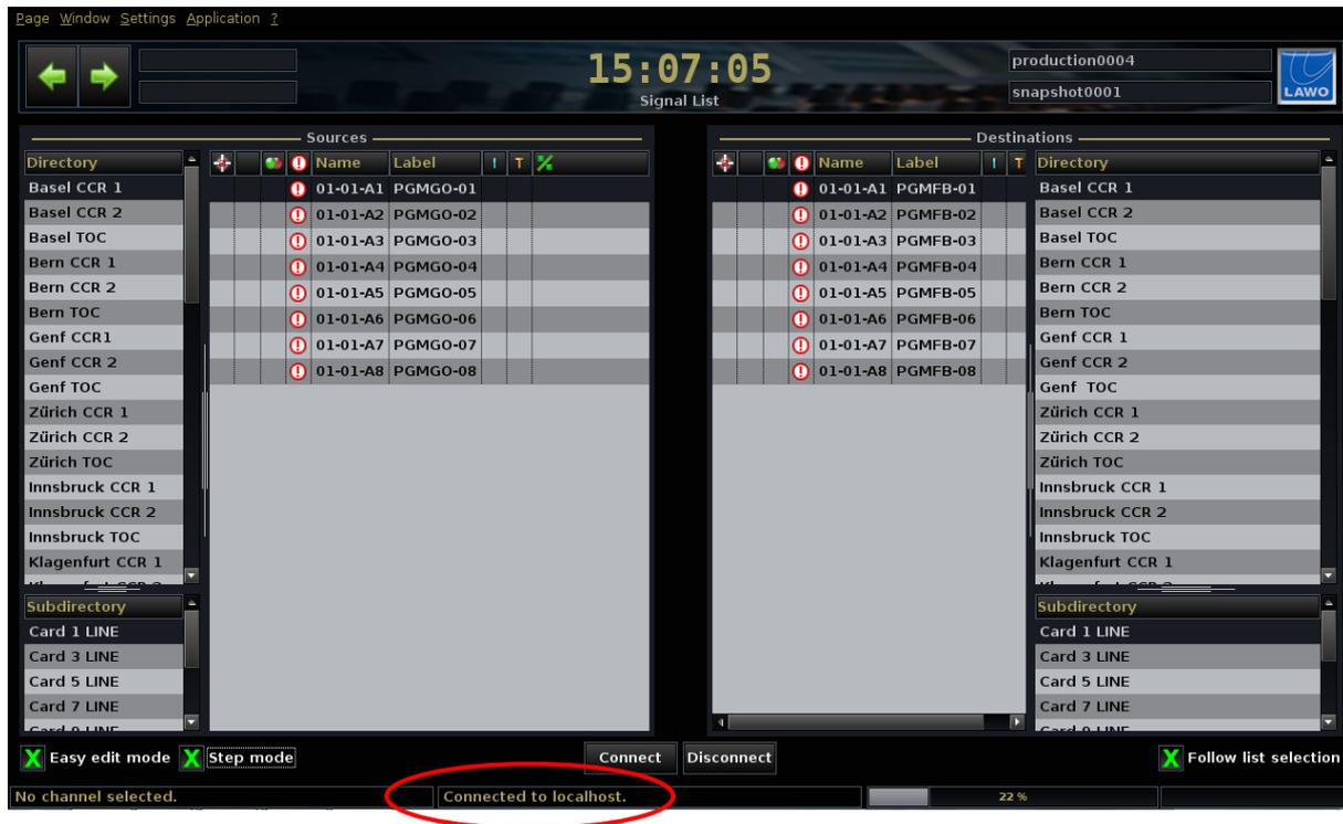
When offline, mxGUI is connected to the “local host”. This means that data is being stored within the “Local Control System”, i.e. on your computer.
