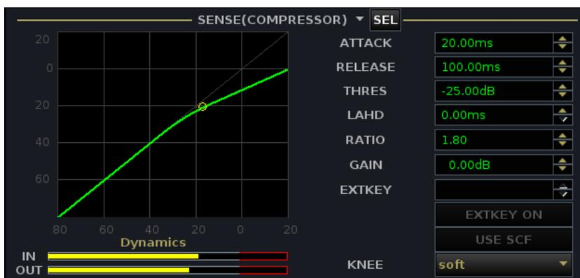
The **IN** and **OUT** meters show the levels to and from the Combi-Dynamics. The **DYNAMICS** metering shows the amount of gain reduction; the **G**, **E** and **C** light in green if the modules are turned on.
