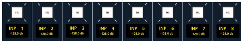
5. Press the **SEL** buttons on the fader strips you wish to switch to Trim
