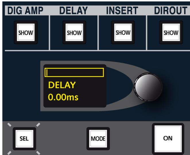
2. Press the DELAY **SHOW** button to assign the controls to the channel delay audio module.
