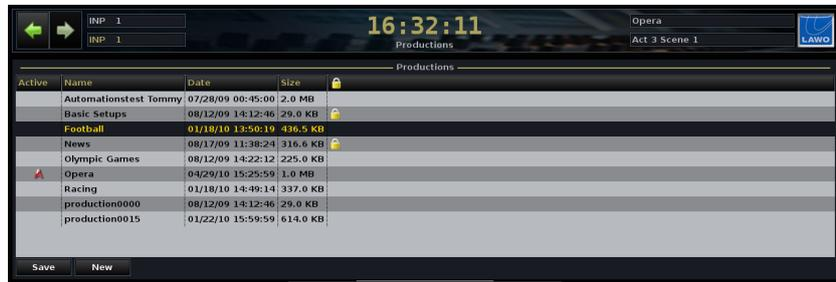
Productions may be recalled at any time, reducing the amount of setup time required before repeat or similar shows. Productions store low level settings, such as the DSP configuration, SRC settings, **System Settings** display options and **Metering** display setup, in addition to snapshots, sequences and automation mixes.
