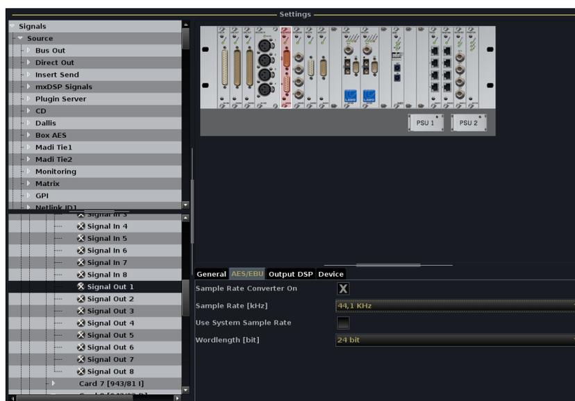
2. To reset the digital output so that it is referenced to system clock, reselect **Use System Sample Rate**.
