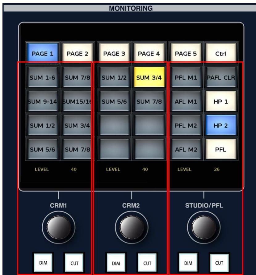
Note that on the classic **mc<sup>2</sup>66**, two monitor outputs (CRM1 and CRM2) are controlled from dedicated panels rather than a touch-screen. The buttons are factory-configured and can be programmed from an identical function set to the MKII **mc<sup>2</sup>66**.
