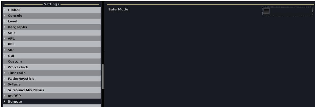
The option determines whether the console may be controlled from a remote device running the Lawo Remote App:
