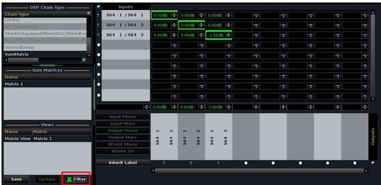
4. To return to all signals, deselect the **Filter** checkbox.
