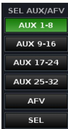
Note that the SEL AUX/AFV options (shown opposite) work exactly as on the console; click **AUX 1-8**, **AUX 9-16**, etc, to switch bank; the **SEL** button must be lit to select the bank. So, in our example above, only the EQ is selected.
