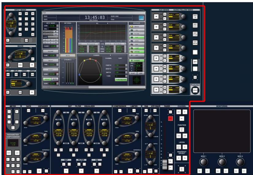
Simply select any channel, by pressing its fader **SEL** button, and then reach out to control any parameter. Remember that the controls are colour coded (MKII mc<sup>2</sup>66 only) making it easy to distinguish the different processing sections.
