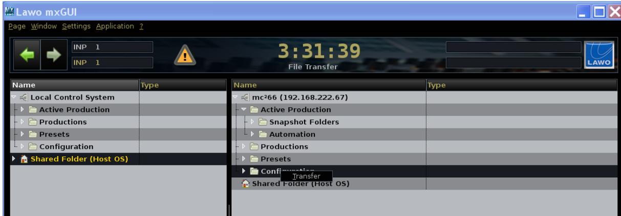
All the configuration files are zipped and transferred to the mxGUI Shared Folder as a single file - **complete\_config**.
