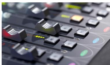
At the bottom of each assigned fader strip, the LAWO backlight is colour-coded to indicate the channel type (MKII mc<sup>2</sup>66 only). This enables you to easily distinguish input channels (white) from sums (red), etc.
