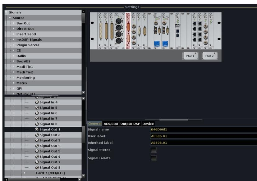
If the selected output is routed from a source, then this field displays the inherited user label and is for information purposes only.
