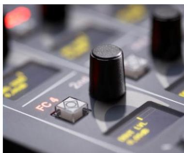
Each of the four free controls can be assigned to key functions for a particular channel. For example, on a presenter's channel it may be important to have direct access to Input gain, the presenter's mix minus send level, the compressor threshold, etc. Whereas, on a music replay channel, it is more important to access L/R Balance, the Direct Output level, etc.
