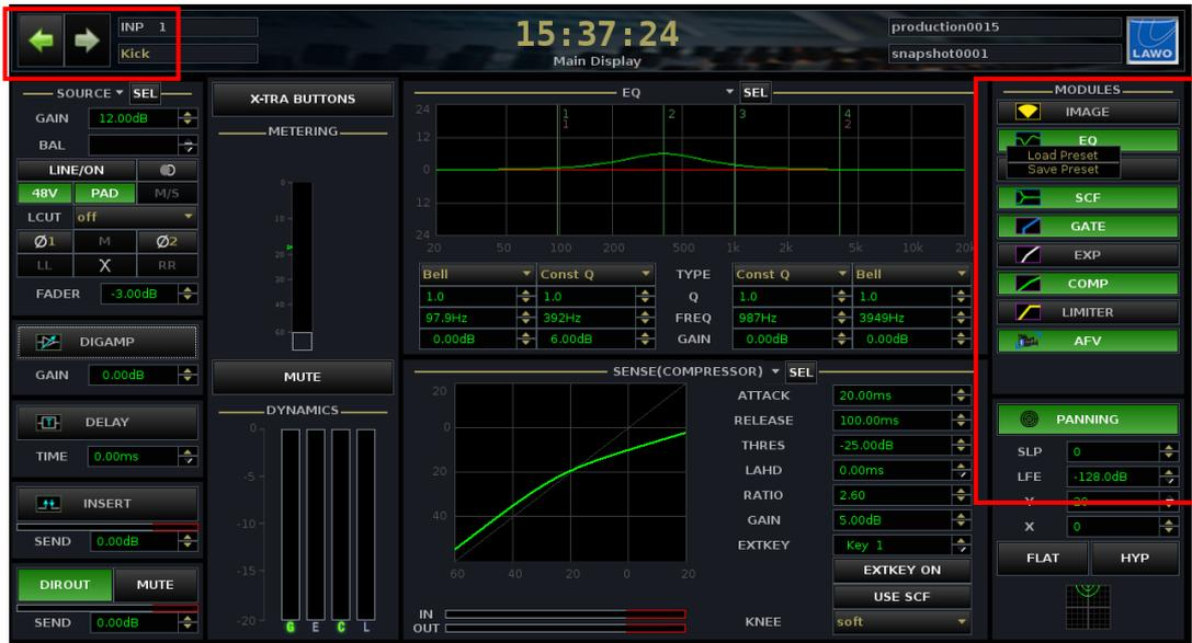
2. Using the trackball and right select button, right-click on the module you wish to save – for example, **EQ**.
