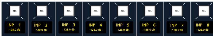
2. Press the flashing fader **SEL** buttons to add channels to the cluster.
