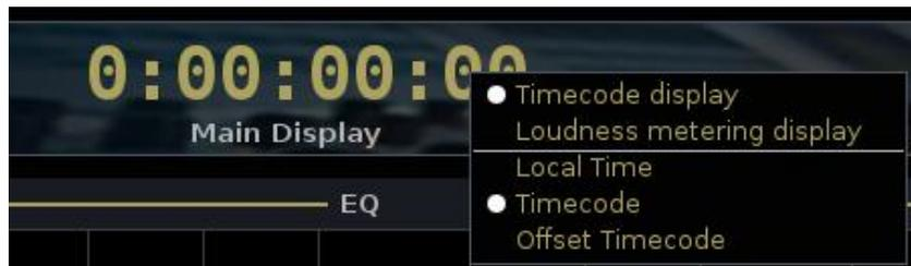
Press PLAY on your machine and check that the timecode on the display follows. If required, you can set a timecode offset and view this on the time display, see Page 542.
