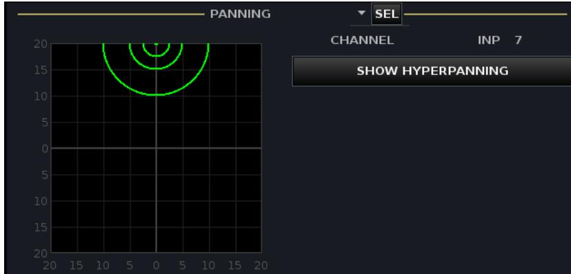
Note that the PANNING module normally follows the channel in access. However, if you are using the **FREEZE** function to lock the joystick to a particular channel, then the Central Control channel and the panning channel may be different. Therefore, the CHANNEL name is always shown on the **Main Display** – in our example, **INP 7**.
