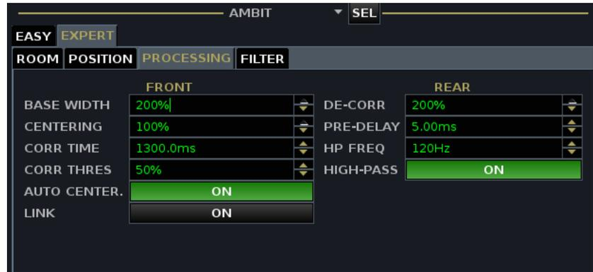
2. When dealing with the FRONT processing parameters, it is best to work with **AUTO CENTER** either on or off:
