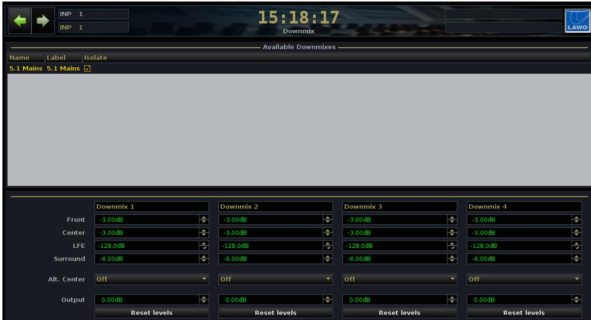
4. Using the trackball or console keyboard, you can adjust the following parameters for Downmix 1 to 4:
