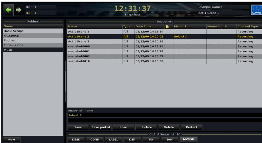
If the list of **Folders** or **Snapshots** is longer than the available window space, focus on the list and use the rotary control on the SCREEN CONTROL panel to navigate up and down the list. You can also resize the windows using the trackball and/or use the on-screen scroll bars.
