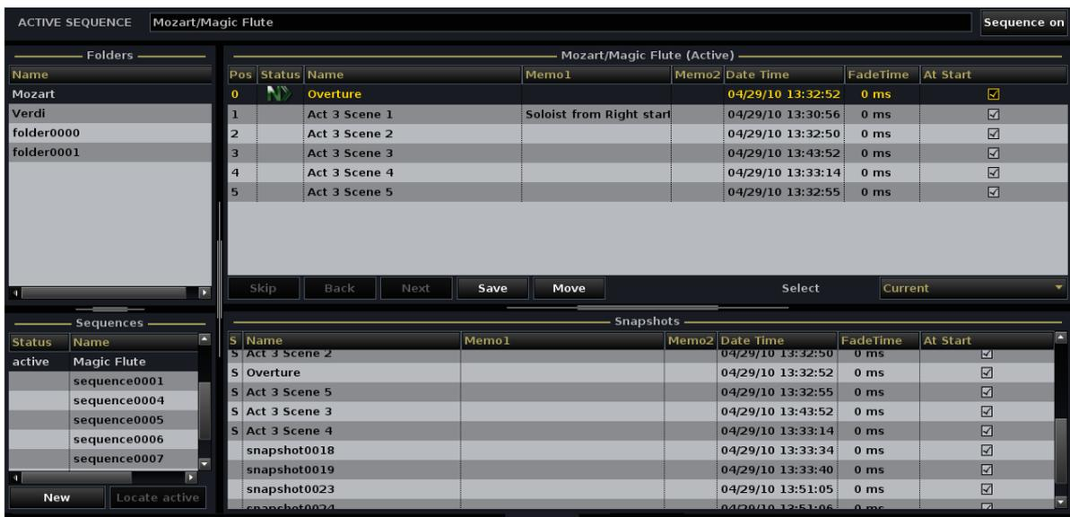
The screenshot shows the 'Sequences' display interface. At the top, the 'ACTIVE SEQUENCE' is 'Mozart/Magic Flute'. Below this, there are two main sections: 'Folders' and 'Sequences'. The 'Sequences' section is active, showing a list of sequence items with columns for Pos, Status, Name, Memo1, Memo2, Date Time, FadeTime, and At Start. The 'Snapshots' section is also visible below the main list.
