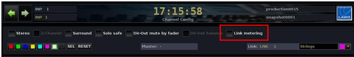
Each channel within the link group now meters signal level for the first 8 channels of the link.
