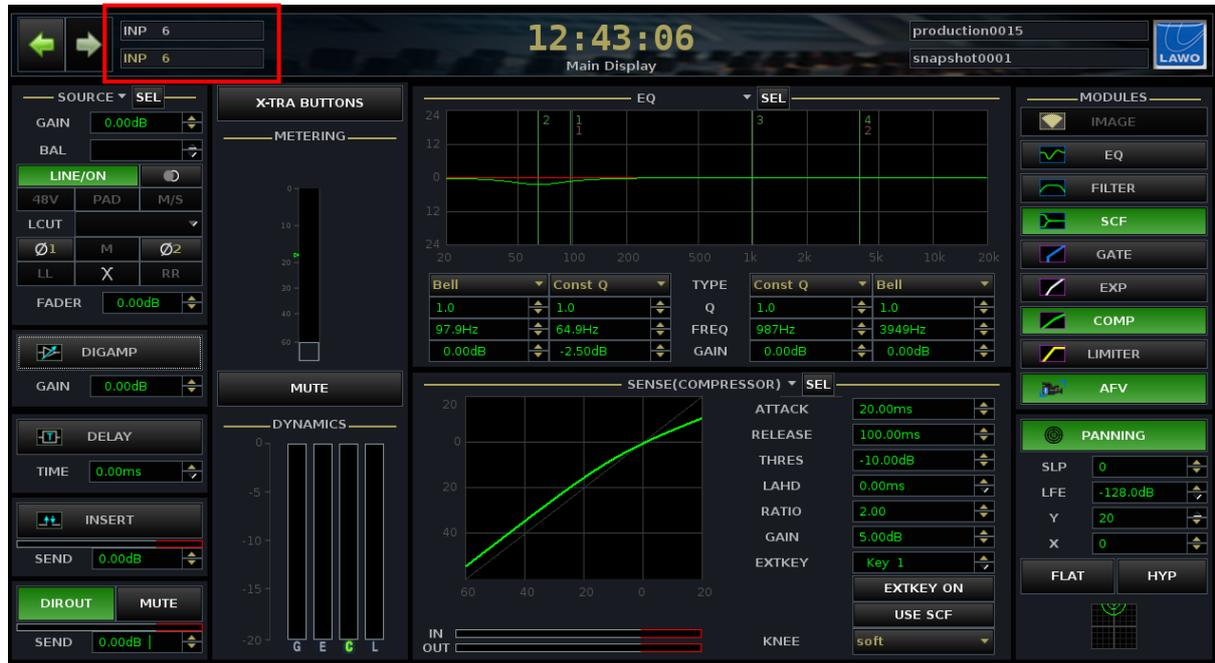
The display is divided into the same sub sections as the Central Control Section front panel. As you adjust controls, the display updates to reflect your settings. In addition, you can change parameters from any of the screen buttons. Green buttons indicate that a section or option is active (ON); on the right of the display, you can see the on/off status for all **MODULES** on the channel.
