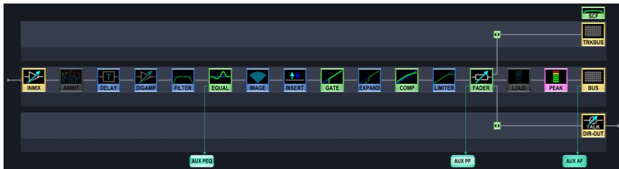
**IN MIX** – channel input gain, phase and stereo input control.
