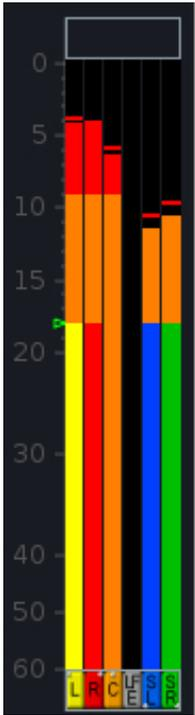
The **Channel** display, above each channel section, includes dedicated metering for every fader strip. On the central control screen, the **Main Display** meters signals at other points such as the insert send, direct out and dynamics modules. And the **Metering** display provides four pages of assignable meters for an overview of key signals.
