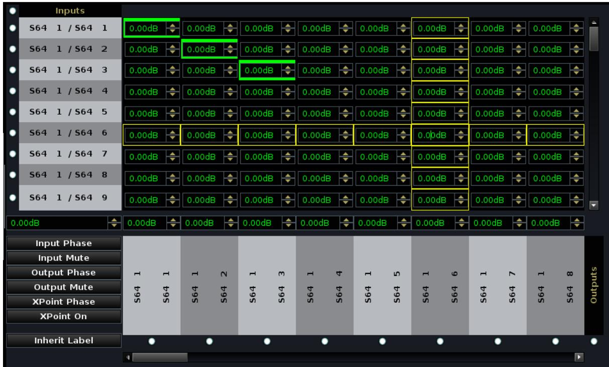
In our example, inputs 1 to 64 run down the left hand side, and outputs 1 to 64 across the bottom.
