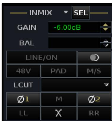
Note that when a fixed gain analogue input is routed to a channel, the **48V**, **PAD** and analogue filter buttons are inactive.
