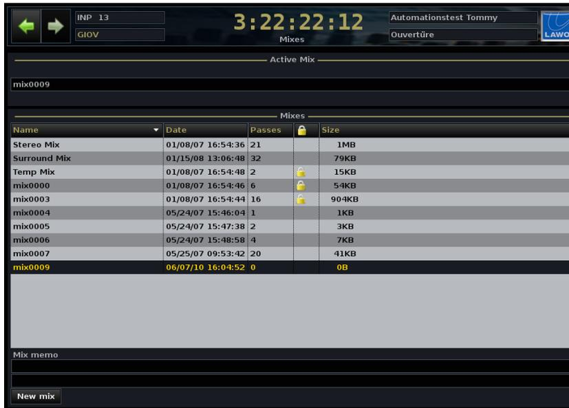
In our example above, a new mix (**mix0009**) was created manually using the new mix function, see Page 484. However, if this is a brand new production, then the system automatically creates a new mix when you turn automation **ON** - **mix0000**.
