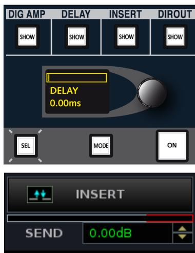
1. Press the **INSERT SHOW** button to assign the rotary controller and buttons to the channel insert module.
