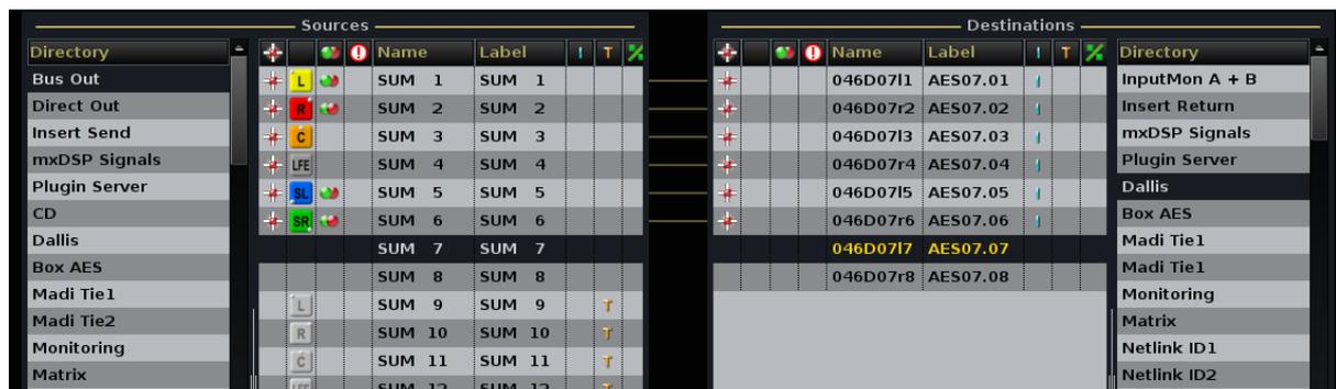
When a snapshot is loaded, any routes made from an isolated source or to an isolated destination are not loaded.
