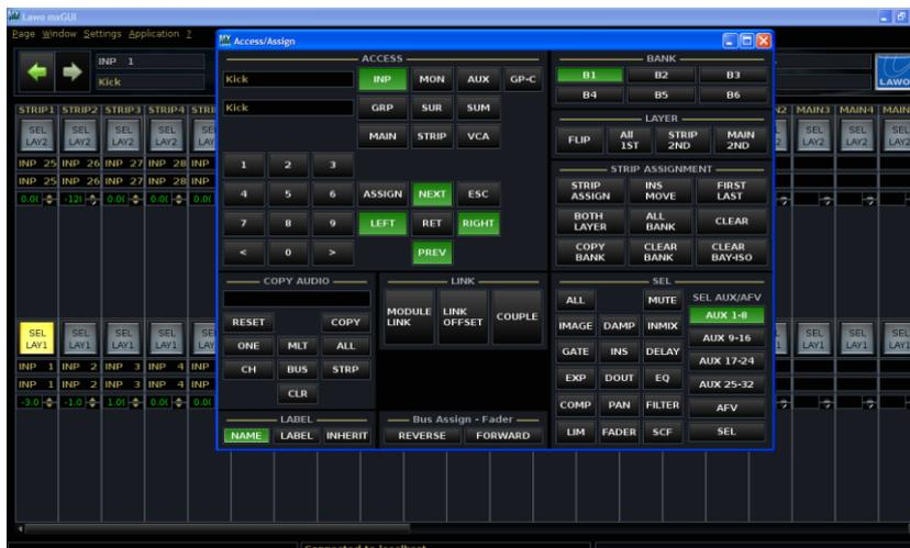
2. Select the source channel you wish to copy from by clicking on the **SEL** button – in our example, fader strip 1, layer 1 (INP 1).
