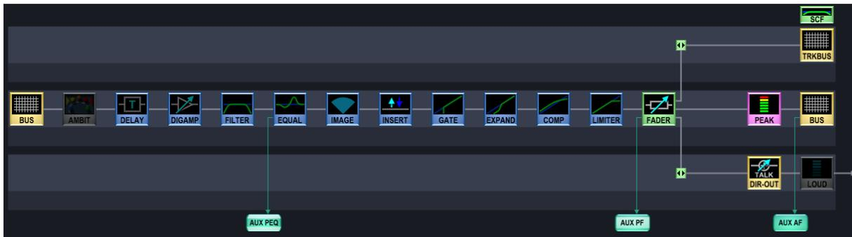
This means that a group can be reassigned to another group or sum, it can feed auxiliary sends, and it has an independently configured insert point, direct output path (and track bus if using a Recording channel DSP configuration).
