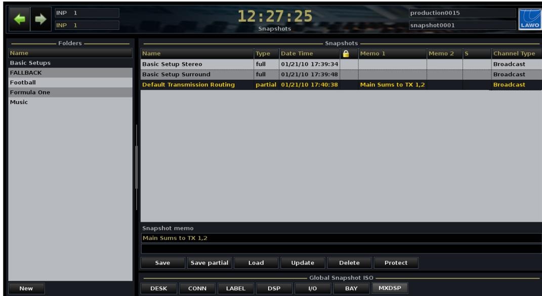
Note that the type of snapshot is marked in the **Type** column to distinguish partial snapshots from full snapshots.
