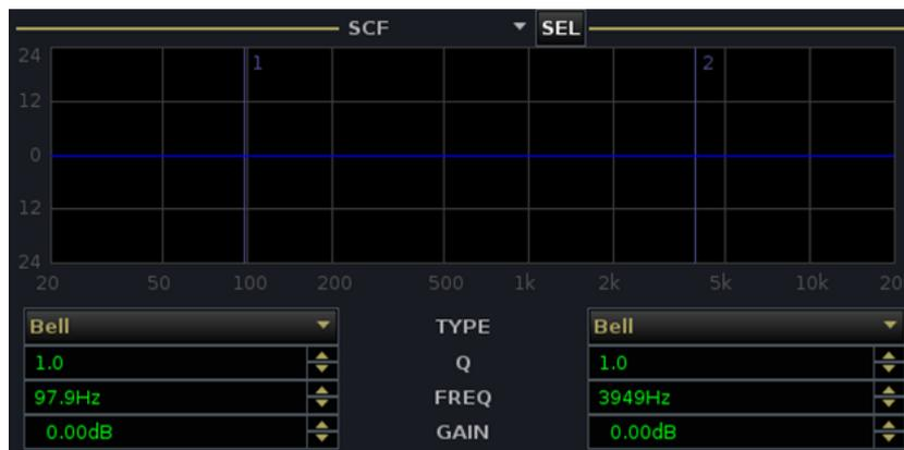
4. Now move over to the SCF/FILTER/EQUALIZER section and use the SCF (Sidechain Filter) controls as described on Page 219 to process the sidechain signal.
