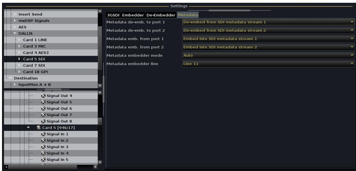
The SDI module offers 2 metadata ports according to SMPTE RDD-2008. This allows embedding, de-embedding and transport of two independent Dolby metadata streams alongside with the video. The streams can be accessed via two D-Sub connectors at the front panel.
