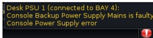
In the mc<sup>2</sup>66, the bay server to the right of the GUI display usually contains the direct connection to the console's external PSU. In our example, this is bay 4 (shown above).
