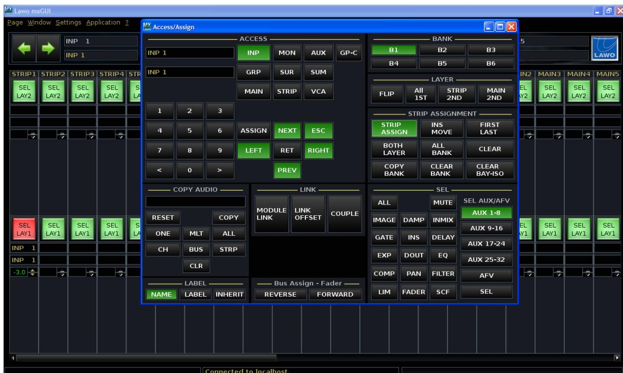
6. Deselect the **STRIP ASSIGN** button and minimise the **Access/Assign** window.
