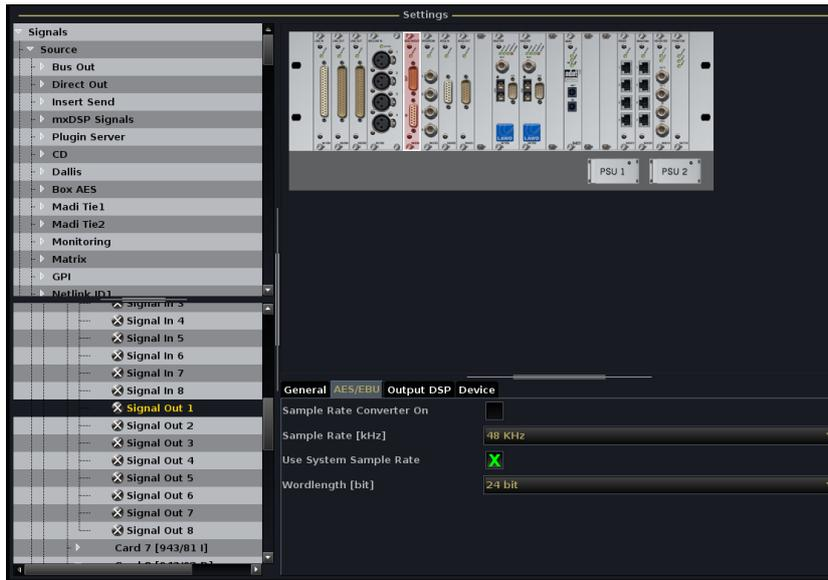
These parameters only appear when an output signal from a AES/EBU card is selected.
