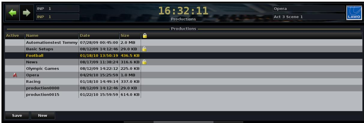
2. To delete the production, press the **DELETE** soft key, or press the right select trackball button and choose **Delete** from the drop-down menu options.
