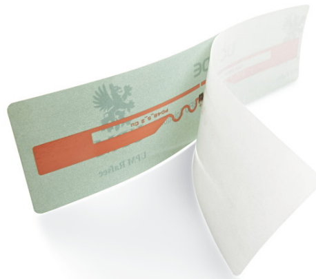
(b) a UHF RFID self-adhesive label
