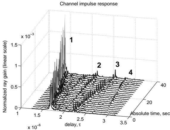
Fig. 3. Measured channel impulse response (non-stationary behavior).
