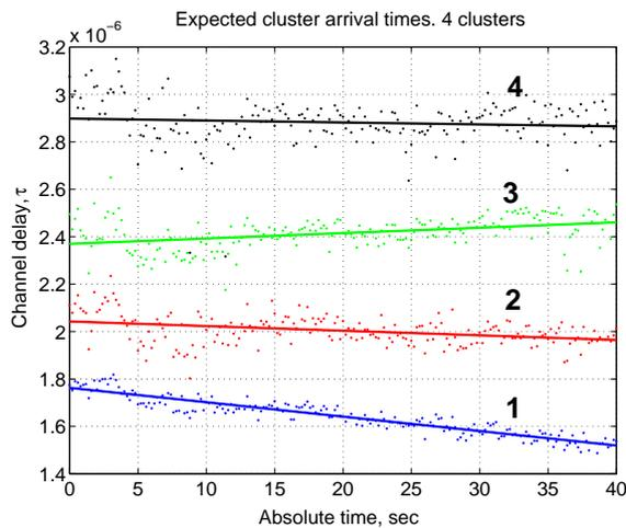
Fig. 4. Expected arrival time tracks of four clusters with superimposed linear regression lines.
