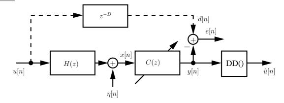
The symbols to be transmitted are  $u[n] \in \{-1, +1\}$ , originate from a stationary process, have zero mean, and are uncorrelated with each other  $E\{u[n]u[n-m]\} = 0, \forall m \neq 0$ . The channel noise  $\eta[n]$  is white, stationary, and uncorrelated with the data  $E\{\eta[n]u[n-m]\} = 0, \forall m$ . H(z) is the discrete-time FIR model of the communication channel, C(z) is an FIR equalizer, and the decision device (DD) is
