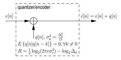
(a) For a process u[n] with a general auto-correlation sequence  $r_{uu}[k]$  and a given quantization noise variance  $\sigma_q^2$ , derive the design equation for an Nth-order (i.e., N coefficients in C(z)) MSE-optimal closed-loop predictor in matrix/vector notation. Hint: to start with, reduce the signal flow graph to the essentials (inputs u[n] and  $q[n] \Rightarrow$  output e[n]).
