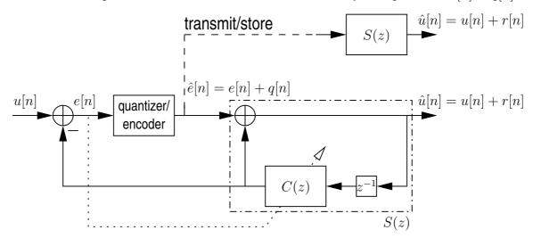
For our calculations, we use the following quantizer/encoder model, and we **assume** u[n]and q[n] to be uncorrelated with each other.  $\Delta_q$  is the quantization cell size, and R is the average bit rate in bits/sample of the lossless encoder-decoder pair (not shown in the figures).
