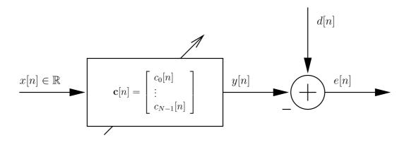
The auto-correlation sequence of x[n] and the cross-correlations between x[n-k] and d[n] are assumed to be known (we can build the auto-correlation matrix  $\mathbf{R}_{\mathbf{xx}}$  and the cross-correlation vector  $\mathbf{p}$ ). The following adaptation rule (*coefficient-leakage gradient search*) is used to adapt  $\mathbf{c}[n]$
