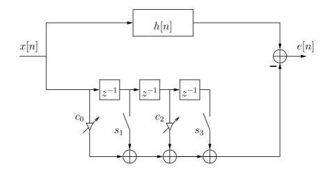
(a) Both switches are open. Determine the MinMSE solution for the two coefficients  $\mathbf{c} = [c_0, c_2]^{\mathsf{T}}$  for a general auto-correlation sequence  $r_{xx}[k]$ .
