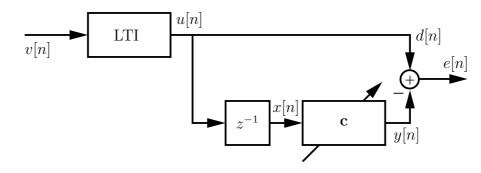
The first 3 samples of the auto-correlation sequence of u[n] are given as  $r_{uu}[0] = 1.0$ ,  $r_{uu}[1] = 0.\overline{5} = \frac{5}{9}$ , and  $r_{uu}[2] = 0.3\overline{7} = \frac{17}{45}$  where the bars denote repeating decimals.
