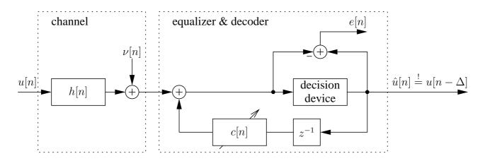
The symbols to be transmitted are  $u[n] \in \{-1, 1\}$ , which occur with the same probability. Consecutive symbols can be assumed to be uncorrelated. Also the channel noise  $\nu[n]$  is uncorrelated with the data u[n-k]. The decision device returns the sign of its input signal (zero is regarded as a positive number). The channel is given as
