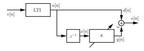
The first 3 samples of the auto-correlation sequence of u[n] are given as  $r_{uu}[0] = 1.0$ ,  $r_{uu}[1] = 0.\overline{5} = \frac{5}{9}$ , and  $r_{uu}[2] = 0.3\overline{7} = \frac{17}{45}$  where the bars denote repeating decimals.
