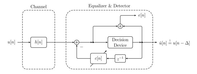
The symbols to be transmitted are  $u[n] \in \{-1, 1\}$ , which occur with the same probability. Consecutive symbols can be assumed to be uncorrelated. The decision device returns the sign of its input signal (zero is regarded as a positive number). The channel is given as
