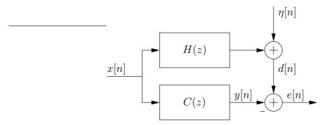
The signal x[n] with zero mean and variance  $\sigma_x^2 = 10$  is used to identify the system H(z) with the impulse response  $h[n] = 0.5\delta[n] - 0.3\delta[n-1] + 0.1\delta[n-2]$ . The adaptive transversal filter C(z) has only 2 coefficients  $\mathbf{c} = [c_0, c_1]^T$ . The additive noise  $\eta[n]$  has zero mean and variance  $\sigma_{\eta}^2 = 0.2$  and is **not fully uncorrelated** with x[n]:
