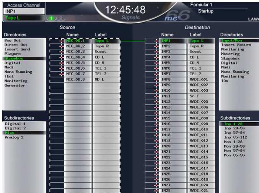
The **Signals** display updates with a green line showing the route between **Mic\_06.1** and **Inp 1**. In addition, the source and destination selections automatically step down to the next entries in the list.
