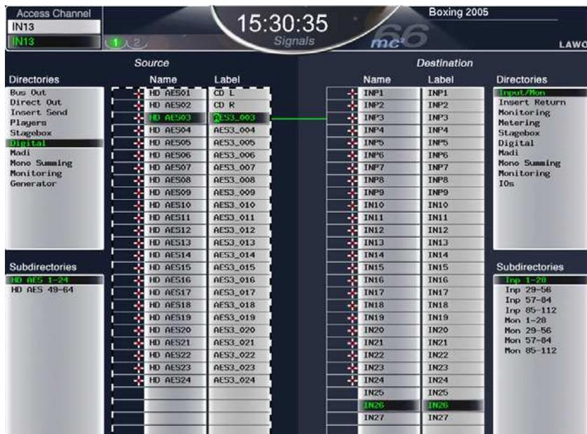
Note that each time you press the **SIGNAL** button you toggle between two pages – **Signals** and **Settings**. The current page is always highlighted at the top of the display – in our example, page 1 of 2.
