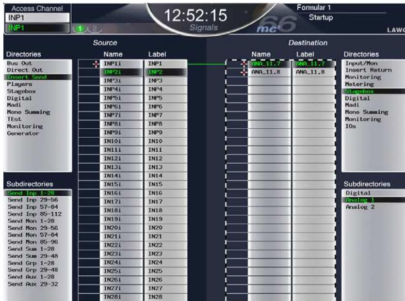
2. Using the trackball or navigation buttons, select the source directory (e.g. **Insert Send**), sub-directory (e.g. **InsSnd Inp 1-24**) and source (e.g. **INP1i**) on the left of the display.
