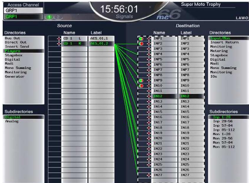
Any source may be routed to any channel, and any output mix routed to any destination. In addition, you may route sources directly to destinations, for example to feed a Mic/Line input to an AES output for archive recording purposes.
