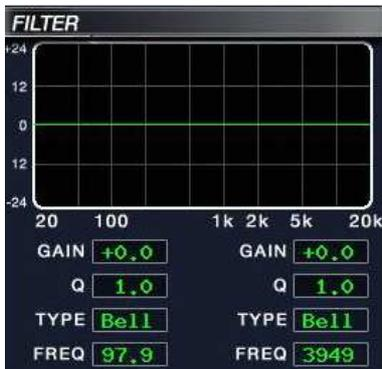
4. Use the FREQ rotary control to set the roll-off frequency for the filter.
