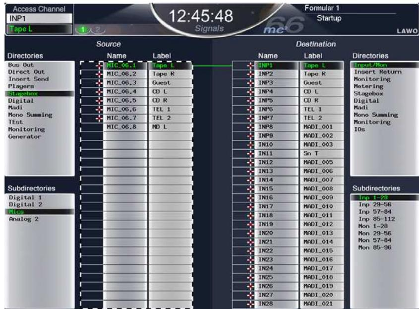
2. Using the trackball or navigation buttons, select the source directory (e.g. **Stagebox**) and sub-directory (e.g. **Mics**) on the left of the display.
