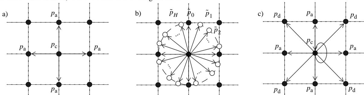
Figure 1: 2D waveguide mesh structures: a) the original mesh with 4 directions, b) the hypothetical version with  $H$  propagation directions, c) the new deinterpolated waveguide mesh, where the new  $\tilde{p}_h$  nodes are spread onto the neighboring nodes by deinterpolation.
