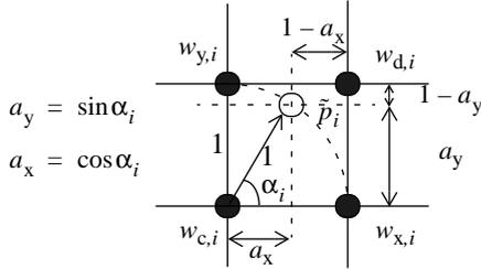
Figure 2: Bilinear deinterpolation coefficients are calculated from this geometry.
