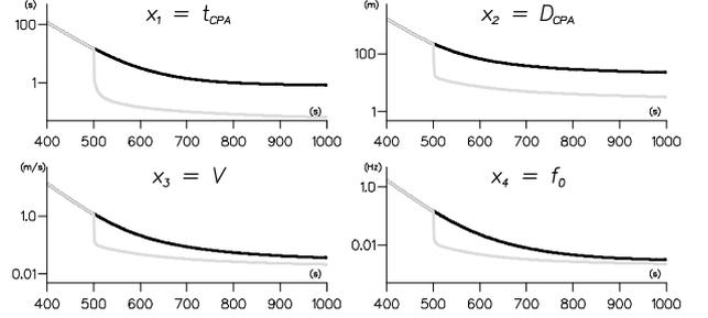
Figure 2. CRLB for one measurement site layout. Acoustic only in black, acoustic and magnetic in grey. The CPA is reached at 500sec. The source is moving at 10m/s, CPA distance is 1.5km, centre frequency is 200Hz. Log scale is used on vertical axis. Input standard deviations are  $\sigma_{k,E/V}=1.0$ ,  $\sigma_{k,D/V}=0.5$  for  $t_k > 500$  and  $\sigma=0.05$ . improved.
