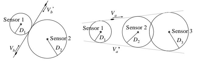
Figure 4. Remarkable configurations and associated ghost solutions.
