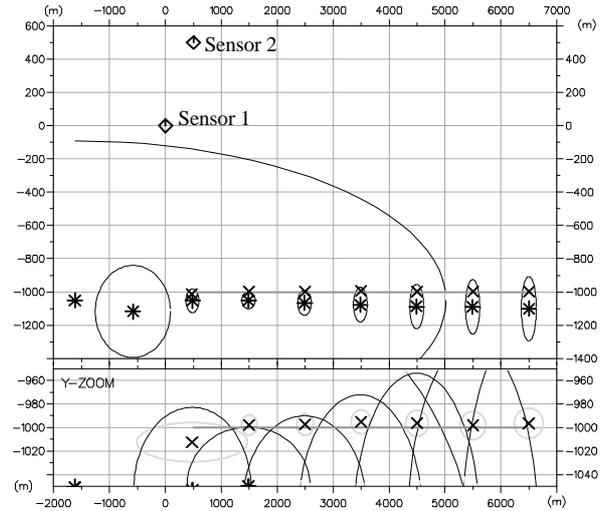
Figure 7. Source localization and two-sigma uncertainty ellipses. It should be strongly emphasize that both axis of each ellipse are scaled identically by the Y-scale. Asterisks (resp. crosses) represent outputs of the Maximum Likelihood estimator strictly based on the past history of acoustic only measurements (resp. of both acoustic and magnetic measurements).
