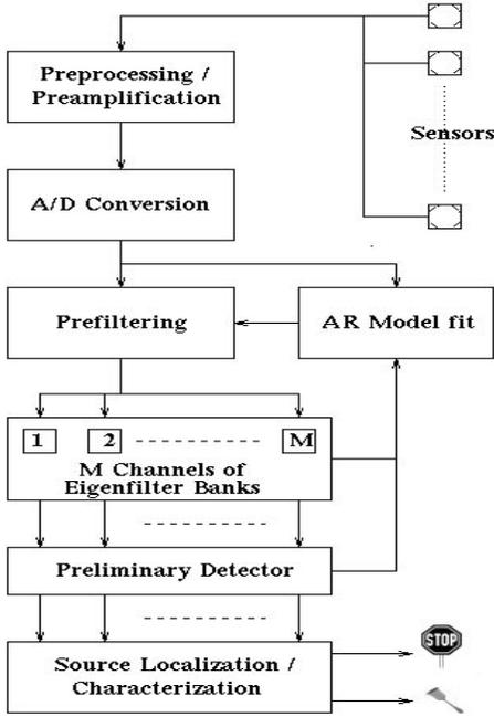
Figure 3. Block Diagram of Proposed Approach
