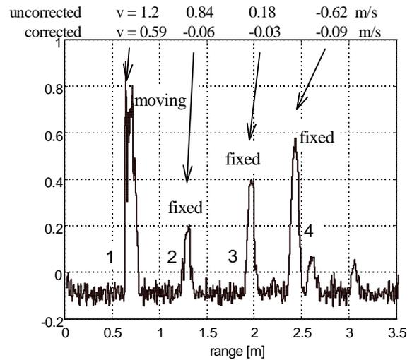
Fig. 5: Echo envelope for 4 targets (1- moving, 2,3,4 -fixed) and their detected velocity before and after applying the correction algorithm
