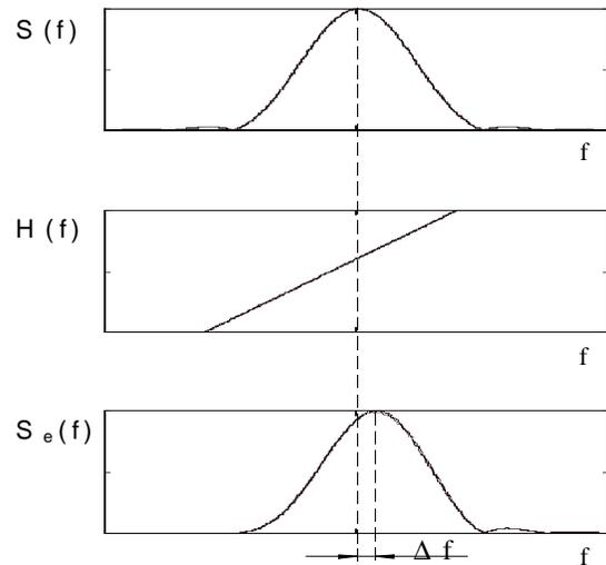
*Fig. 1: Frequency shift due to a nonlinear transfer function*
