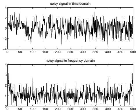
Figure 4: Noisy signal and its Fourier spectrum.
