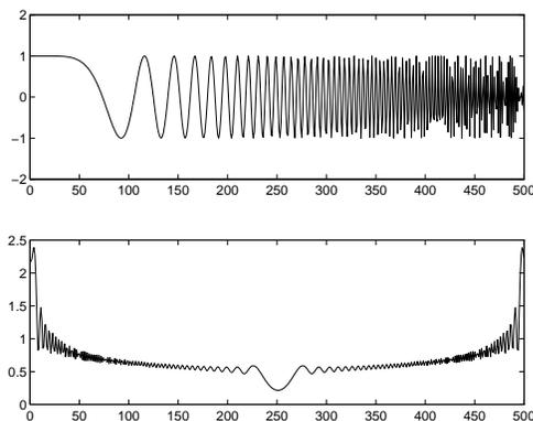
Figure 3: The chirp signal and its Fourier spectrum.
