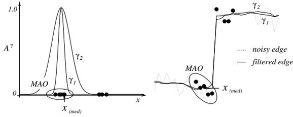
**Figure 3.** Edge preservation property: (left) Assigning affinity measures to observations from a noisy step edge. (right) Noisy (dotted) and median affine filtered edge (solid) for  $\gamma_1$  and  $\gamma_2$ , where  $\gamma_1 < \gamma_2$ . The larger value of  $\gamma$  results in increased smoothing left and right of the edge.
