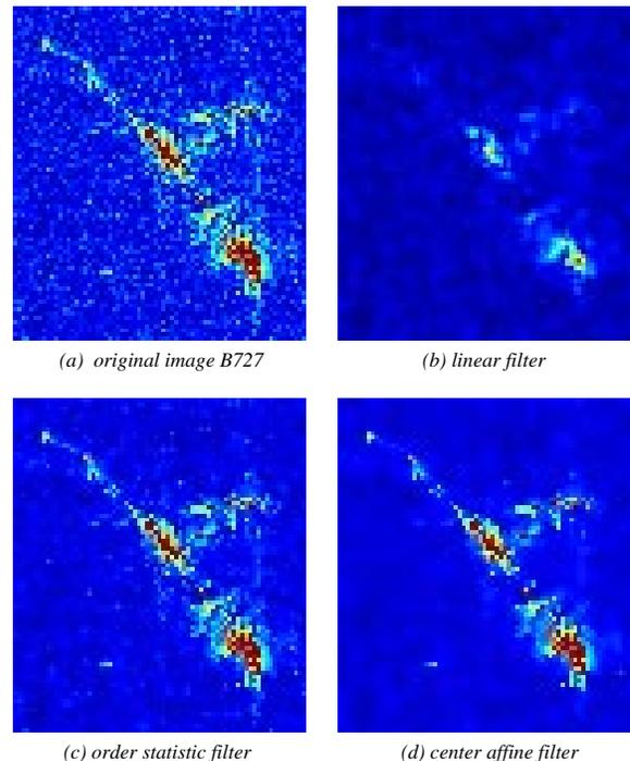
**Figure 5.** Feature enhancing using the center affine filter.
