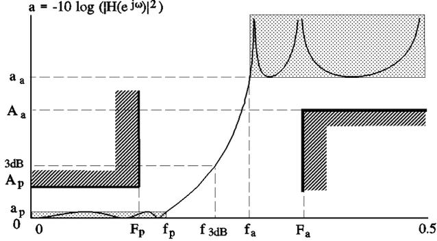
Figure 1. A typical elliptic filter
