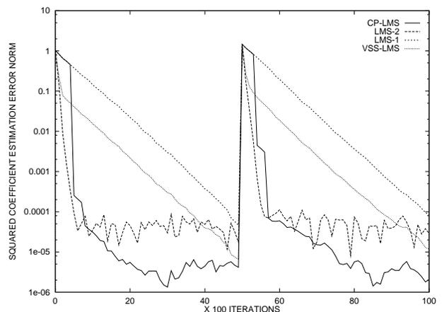
Figure 3. Norm squared estimation error plot
