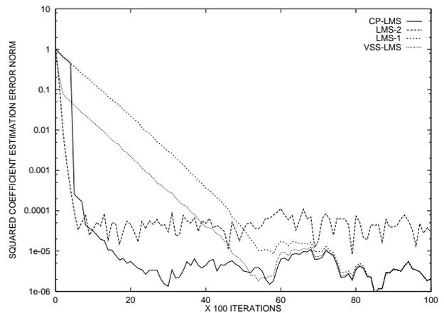
Figure 2. Norm squared estimation error plot
