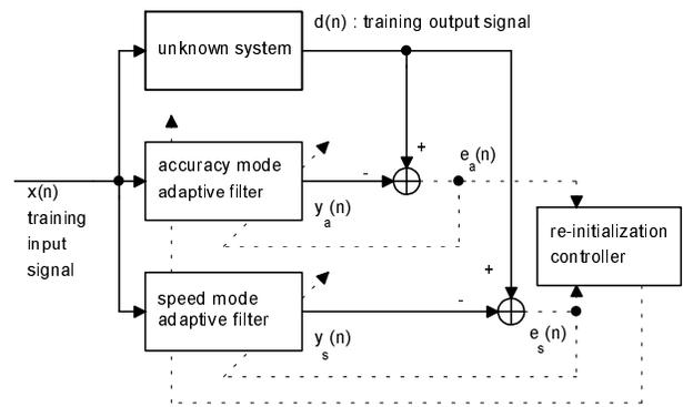
Figure 1. The CP-LMS algorithm block diagram
