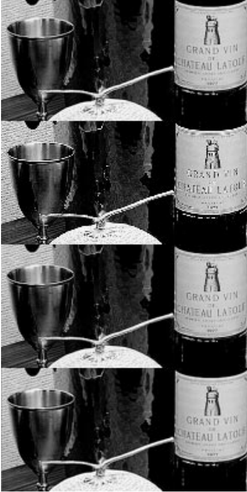
Figure 4: Reconstructed JPEG images at a quarter resolution. From top to bottom: proposed method; no filter; 4 \times 4 averaging; and 21 \times 21 Hamming filter.
