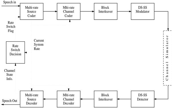
Figure 1. MRC-CDMA schematic block diagram
