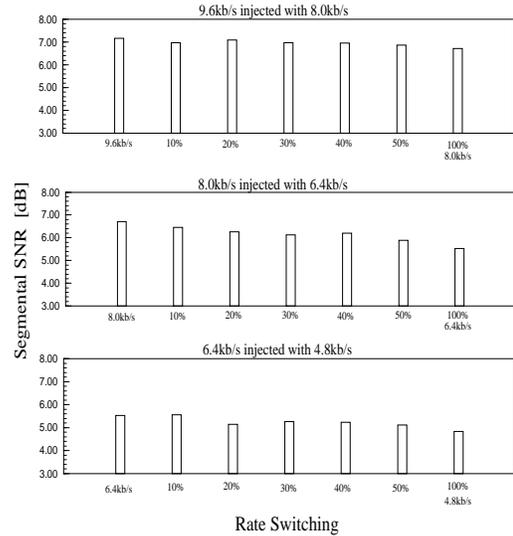
Figure 2. Performance of multi-rate codecs with rate switching
