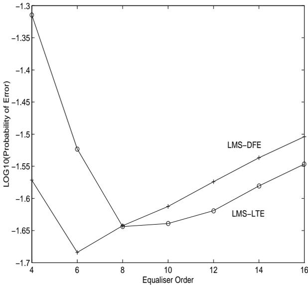
Figure 4: Equaliser order dependency for the LMS LTE and LMS DFE on channel 2 with a fade rate of 2 Hz and a signal-to-noise ratio of 20 dB. The equaliser order corresponds to  $M - 1$  for the LTE and  $M_f + M_b - 1$  for the DFE. For the LTE, the delay is set to  $(M - 1)/2$ . For the DFE,  $M_b$  is fixed on  $M_b = 2$ .
