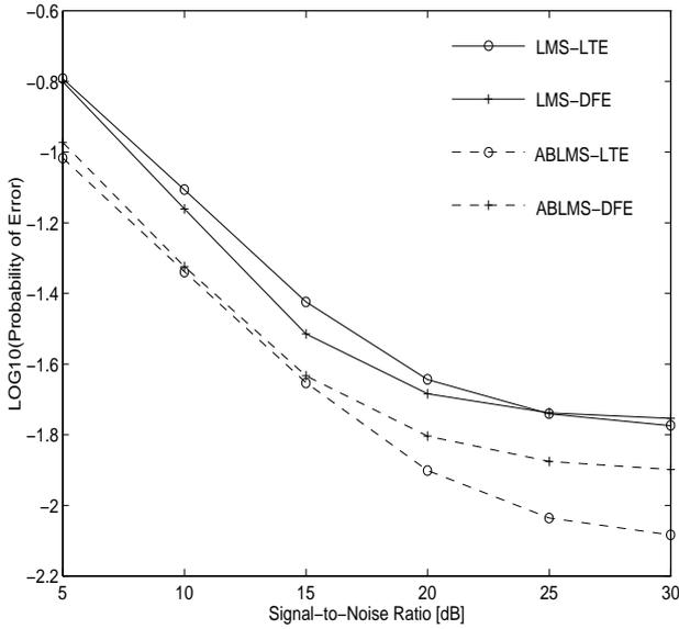
Figure 3: Bit error rate performance against additive noise on channel 2.
