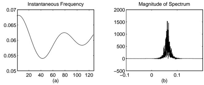
Figure 1. A Typical Modulating Signal Segment (real part) and the Signal Spectrum
