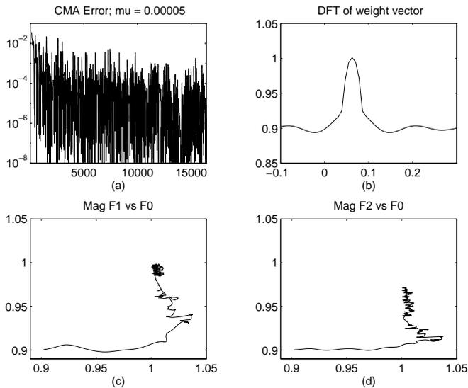
Figure 3. Typical Convergence Behavior for a CMA-directed Filter with a Noise-loaded FM Input
