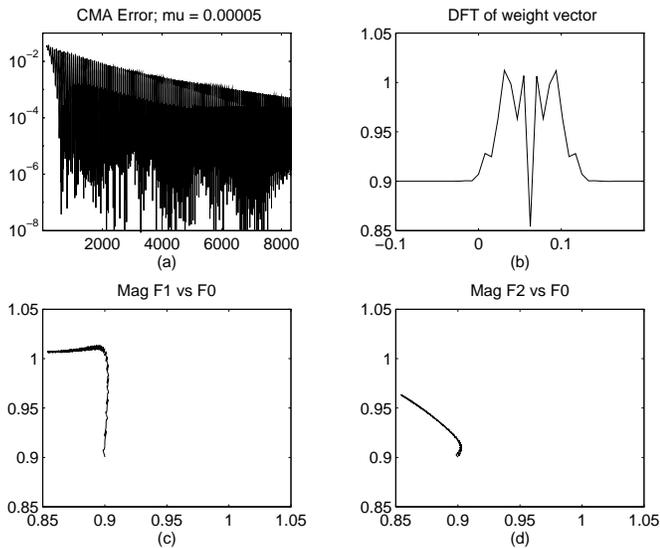
Figure 5. Misconvergence of CMA for Modulating Signal Composed of two Sinusoidal Signals at Frequencies of  $1/N$  and  $3/N$ .
