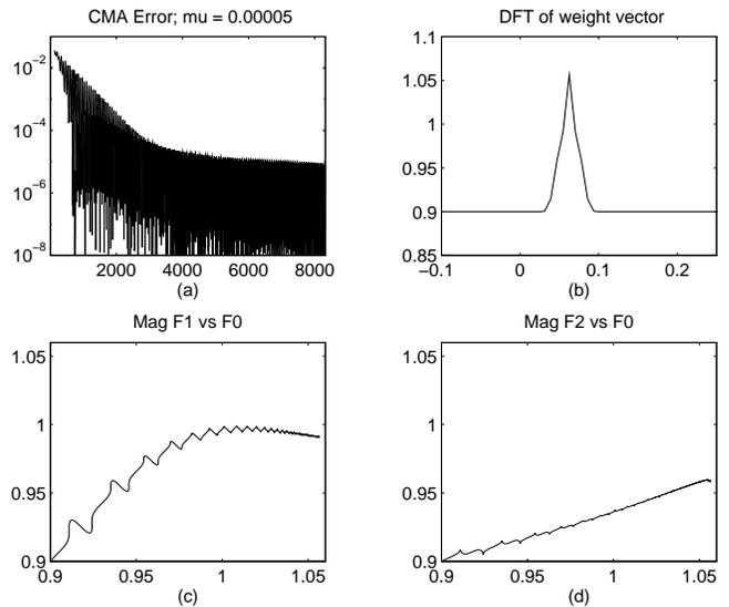
Figure 4. Convergence of CMA for Sinusoidal Modulating Signal with Frequency  $1/N$ .
