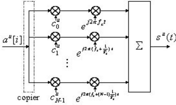
Fig. 2. Transmitter model for MC-CDMA system
