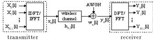
Fig. 1. A block diagram of an OFDM system
