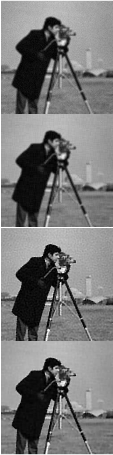
Figure 2: From top to bottom: (a) Image blurred with the 5 \times 5 uniform blur PSF, SNR=20dB, (b) result of applying the denoising algorithm to the image in (a), (c) result of applying the deblurring algorithm to the image in (a), (d) result of applying the deblurring algorithm to the image in (b).
