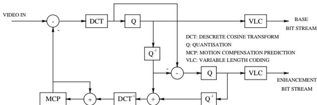
Figure 1. Block diagram of SNR scalable coder
