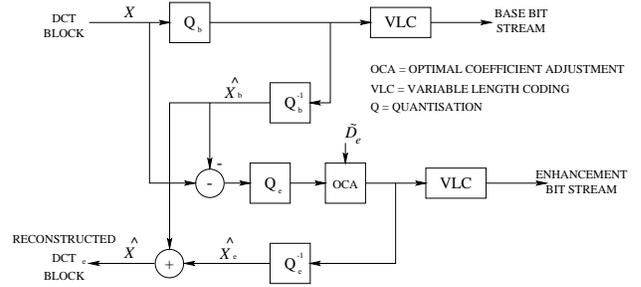
**Figure 2. Block diagram of optimised SNR quantisation stage**
