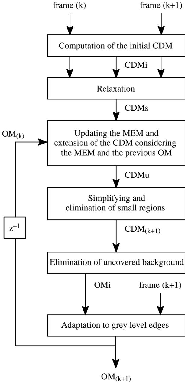
Figure 1: Block diagram of the segmentation algorithm.
