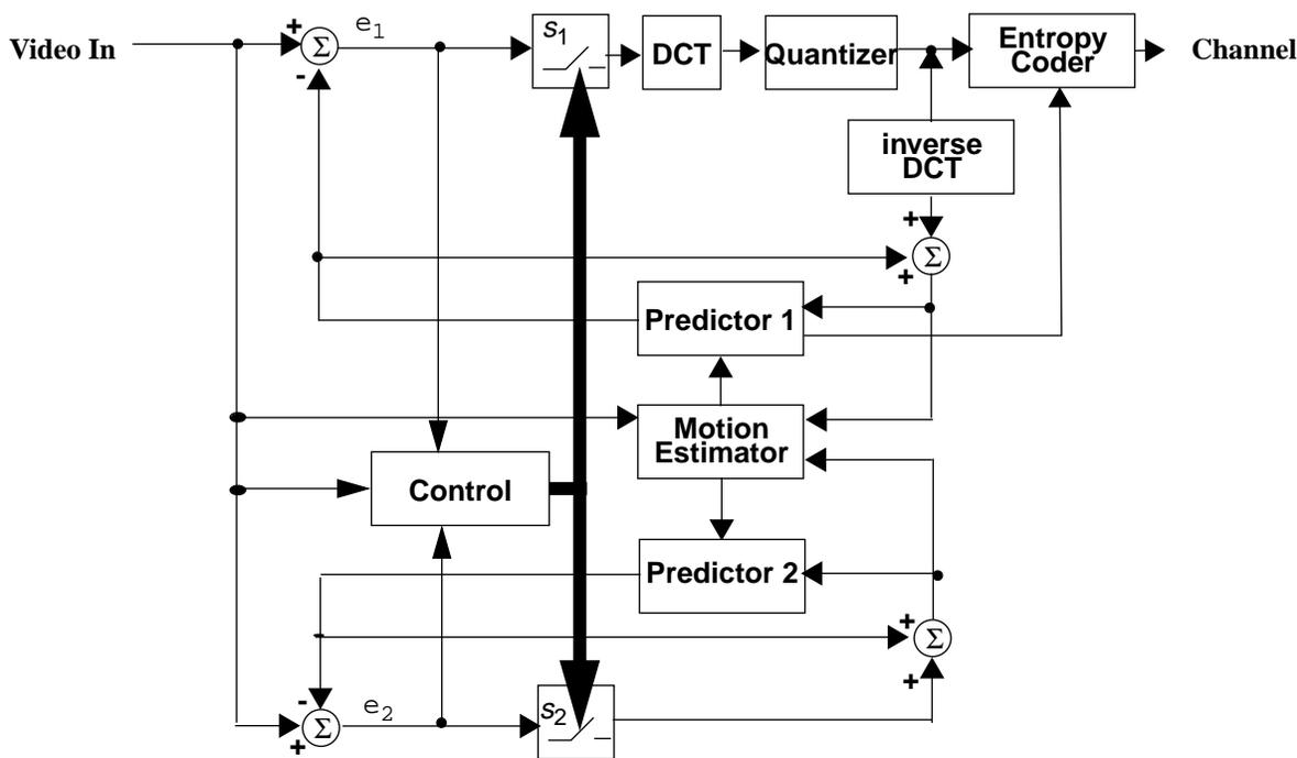
Figure 1: Block diagram of a block-based hybrid coder with a second predictor loop. The switches  $s_1$  and  $s_2$  are operated synchronously by coder control. Predictor 1 and Predictor 2 use the same prediction mode for each block.
