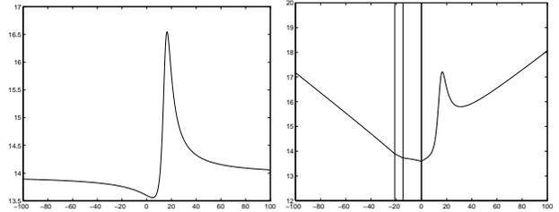
Figure 2: Left: Illustration of the data part of the 1-D criterion:  $\mathcal{J}_{\text{ML}}(\mathbf{x} + \mathbf{x}_i)$  (rational fraction). Right: Illustration of the 1-D criterion  $\mathcal{J}_{\text{MAP}}(\mathbf{x} + \mathbf{x}_i)$  for  $L_1$  regularization (piecewise rational fraction).
