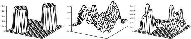
Figure 3: Original object (left) and solution given by the conjugate gradient (center) and by the proposed algorithm (right) after 10 iterations ( $L_{1,1}$  regularization). The object has a relative contrast of 2,  $21 \times 21$  pixels and  $8 \times 8$  data are available with  $\text{SNR} = 20\text{dB}$ .
