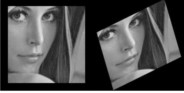
Figure 1. Modelling of 3-D rotations by affine transform. (Left) Original image plane lying on xy -plane. (Right) Projection of the planar object on xy -plane after rotating by (\theta, \alpha, \beta) = (30^\circ, 30^\circ, 30^\circ) using proposed method.
