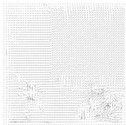
Fig. 2. Motion field obtained for frames 0 and 3 of sequence "Calendar and Train" (caltrain)
