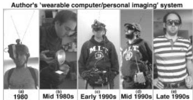
Figure 1: Evolution of author's wearable computer/personal imaging invention. Large head-mounted CRT and separate inbound and outbound communications antennas of the late 70s were awkward. Author's waist-mounted television of the mid 80s was somewhat more comfortable but not constantly visible. Small viewfinders from consumer video cameras of the late 80s made possible an eyeglass-based system which later evolved toward author's current embodiment built into ordinary eyeglasses.
