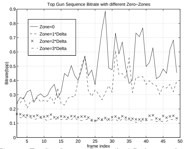
Figure 4: Top-Gun Sequence Bitrate (bpp) Performance for Multiplierless PR-QMF Codec.
