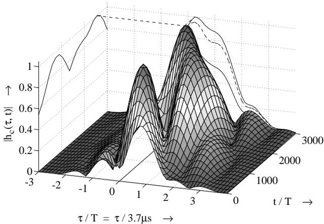
**Figure 4:** Impulse response of a *Bad Urban* channel
