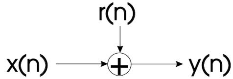
Figure 2: System model for the analysis of cumulant estimation errors
