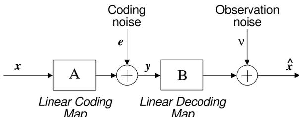
Figure 1. Codec using Principal Component Analysis with noisy representation.
