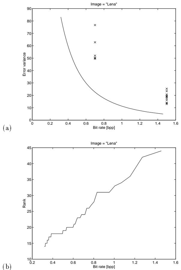
Figure 3. (a) Rate-distortion plot for the NPCA-optimal 64-bank filter using the  $256 \times 256$  image "Lena". As a comparison we show the corresponding R-D points obtained in [9] for different filters (points marked by 'x'). (b) The optimal rank as a function of the bit-rate.
