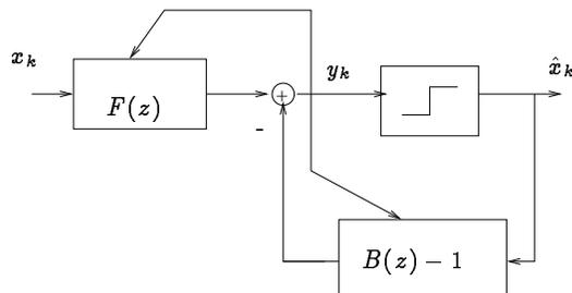
Figure 1: Schematic of CMA-DFE
