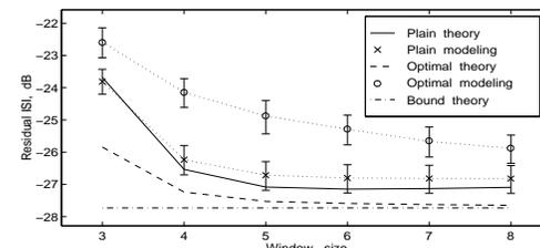
Fig.3. Residual error versus the analysis window size  $N$ .
