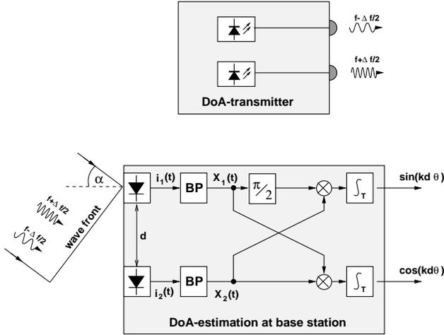
**Figure 3.** Transmitter (terminal) and receiver (base station) for DoA-estimation ( $k = 2\pi/\lambda$ ,  $\theta = \sin(\alpha)$ ).
