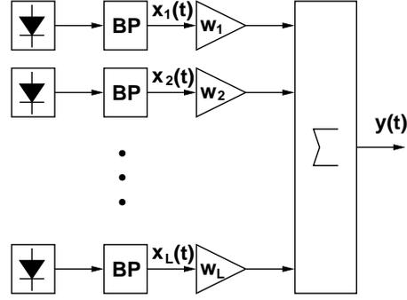
Figure 5. Beamformer with  $L$  elements
