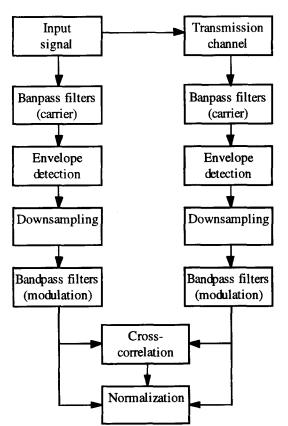
Although the use of IIR filters in the carrier bandpass filters results in a computationally more efficient realization for given stopband attenuation, it is advisable to implement the filters either as equal-length FIRs or, if IIR implementation is attempted, they should be used as dual-pass linear-phase filters in order to keep the modulation envelopes of all the carrier and modulation bands time-aligned.
