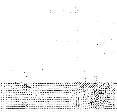
Fig. 2. Motion field obtained for frames 0 and 3 of sequence "Calendar and Train" (caltrain)
