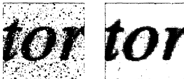
Figure 3. Smoothing of blurred image plus impulsive noise. (Left:) noisy image, and (right:) image smoothed with a 3 \times 3 median filter.
