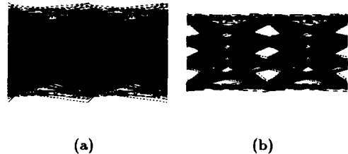
Figure 2: Equalization results of the 16-QAM system. (a) Received signal. (b) Equalized signal.
