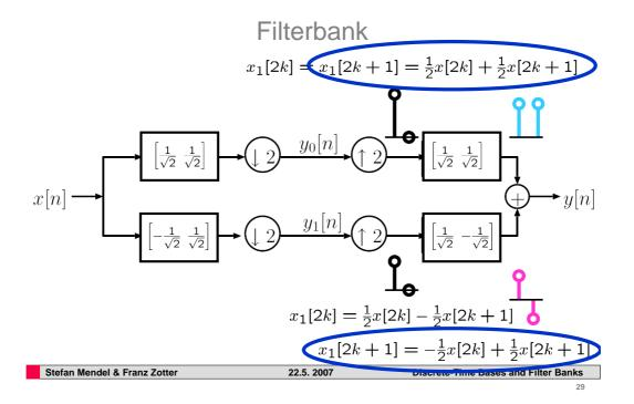
Odd samples  $y[2k+1] = x_0[2k+1] + x_1[2k+1] = (\frac{1}{2}x[2k] + \frac{1}{2}x[2k+1]) + (-\frac{1}{2}x[2k] + \frac{1}{2}x[2k+1]) = x[2k+1].$
