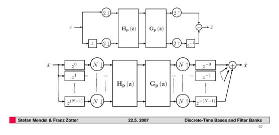
Of course, like in the modulation domain before, we can extend the notations for N-channel filter banks. Here, the criteria remain exactly the same, as no re-normalization is involved.
