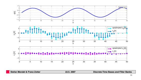
Synthesis filter:  $g_0[n] = \phi_0[n] = (1/sqrt(2) 1/sqrt(2))$ . That means that for a delta impulse we have the response  $\phi_0[n]$ , which is a scaled reproduction of the sample.
