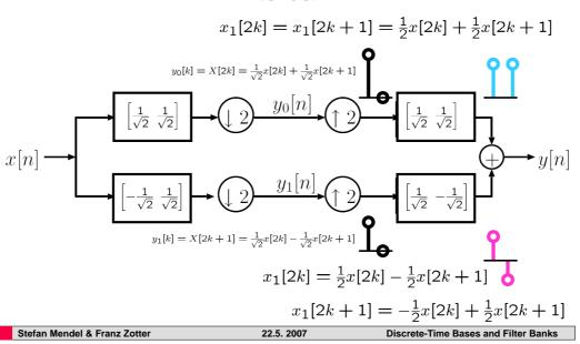
The impulse response of  $g_0$  reproduces a scaled (by 1/sqrt(2)) version of the input sample (since the second sample is zero), whereas  $g_1$  produces the same output, but once time -1.
