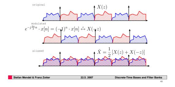
For frequency domain representations of decimated filter banks, we have to do some tricky manipulation, in order to provide sufficient description of "aliasing", i.e. timevariance. A straight-forward way is to build the aliased spectrum obtained from downsampling and expansion by modulation and sum of the original signal spectrum. Mind the re-normalization term deviding by the number of modulated spectra. This normalization is necessary, as downsampling and upsampling scales the signal energy.
