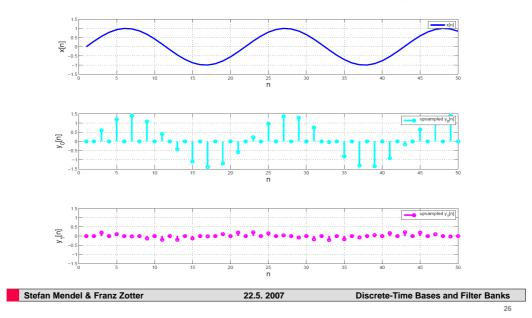
Upsampling by 2: Inserting yeros, i.e., every second sample is zero.
