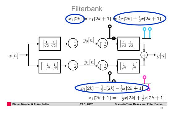
Even samples y[2k] =  $x_0[2k] + x_1[2k] = (\frac{1}{2}x[2k] + \frac{1}{2}x[2k+1]) + (\frac{1}{2}x[2k] - \frac{1}{2}x[2k+1]) = x[2k].$
