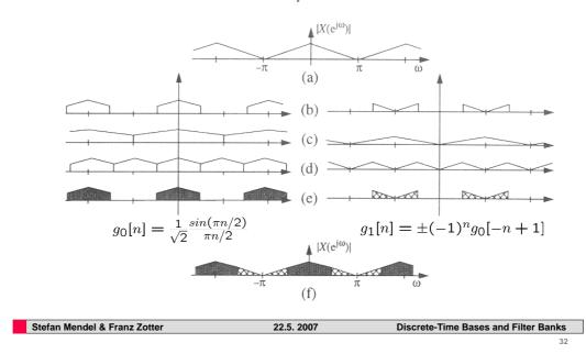
On the left side we see the projection of the input signal x[n] onto the subspace of sequences bandlimited to  $[-\pi/2 + \pi/2]$  (i.e. lowpass) shown in black.
