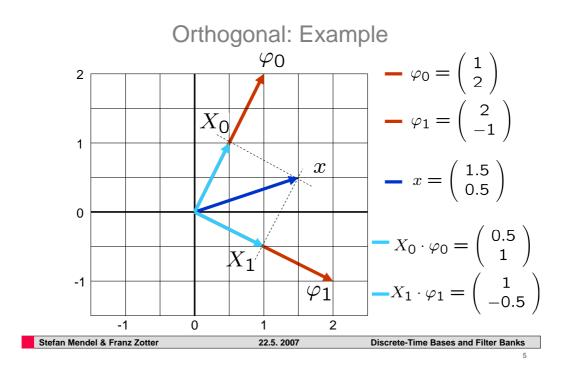
An example for an orhogonal expansion. Note that this expansion is not orthonormal, since the scalar product of  $\langle \varphi_0, \varphi_0 \rangle = 5$  and  $\langle \varphi_1, \varphi_1 \rangle = 5$  are not normalized to 1.
