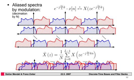
The following slides shall illustrate, how the more general case of decimation by N, as well as the N-channel filter bank can be constructed in the modulation domain.
