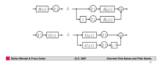
The third way to implement our filter bank is the polyphase domain. While the modulation domain employed filters at the original sampling rate, the polyphase domain more efficiently utilizes the polyphase realizations of decimation and reconstruction filters, we already heard about.
