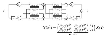
$$\hat{X}(z) = \begin{pmatrix} 1 & z^{-1} \end{pmatrix} \underbrace{\begin{pmatrix} G_{00}(z^2) & G_{10}(z^2) \\ G_{01}(z^2) & G_{11}(z^2) \end{pmatrix}}_{\mathbf{G_{D}}(z)} \mathbf{Y}(z^2)$$
