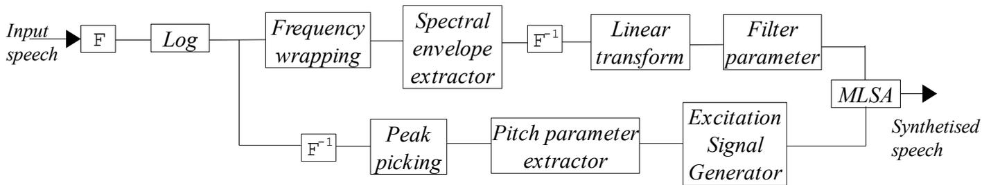
Note that the MLSA filter is used as the speech synthesizer. The filter coefficients are obtained through a simple linear transform from the mel cepstrum which is defined as the Fourier cosine coefficients of the “true” spectral envelope of the mel log spectrum.
