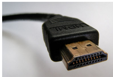
Abb 4-12: HDMI-Stecker [D-Kuru on Wikipedia]
