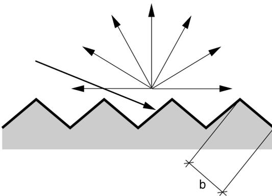
$\lambda \approx b$ : The reflected wave can be reflected in any direction, which increases the diffusivity of a sound field.
