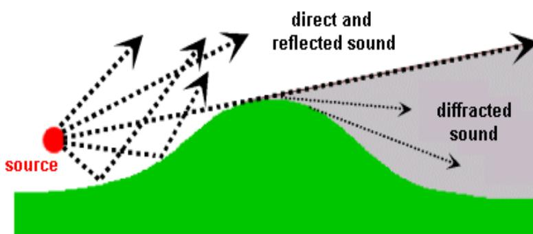
*Picture 1.7 :Diffraction on an obstacle*
