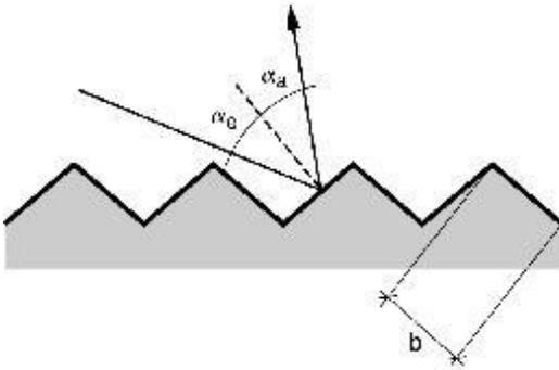
$\lambda < b$  : Each sub surface reflects the wave on it's own according to the geometric reflection lemma  $\alpha_e = \alpha_a$
