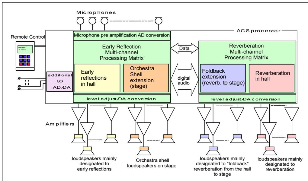
Figure 5.9: ACS Block Diagram [ACS, 2009].
