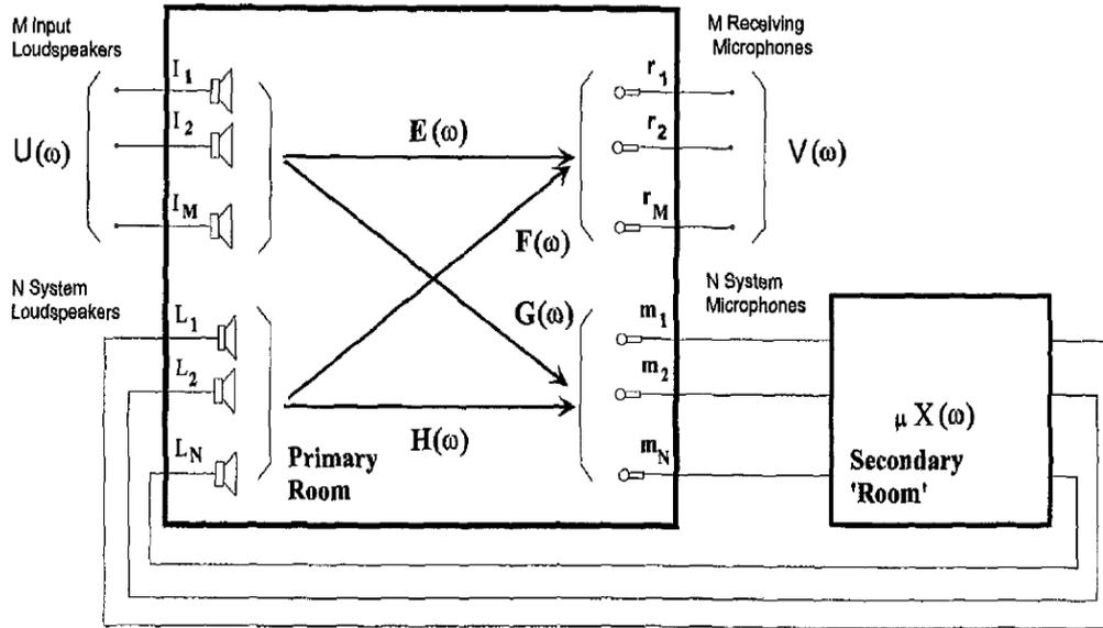
Figure 5.12: Block diagram of the VRAS [Poletti, 1996].
