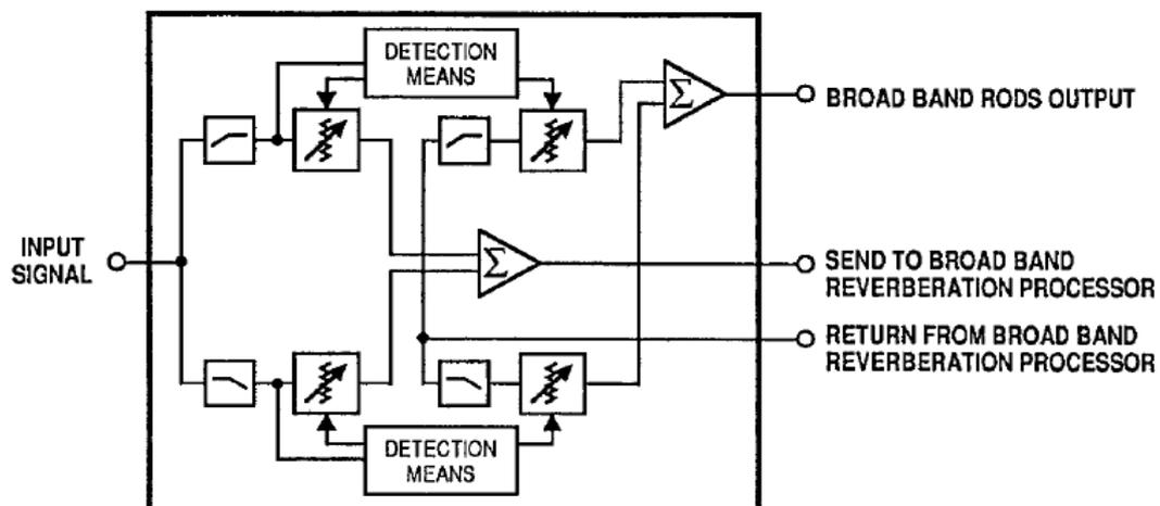
Figure 5.5: *Simplified RODS Schematic* [Jaffe, 1992].
