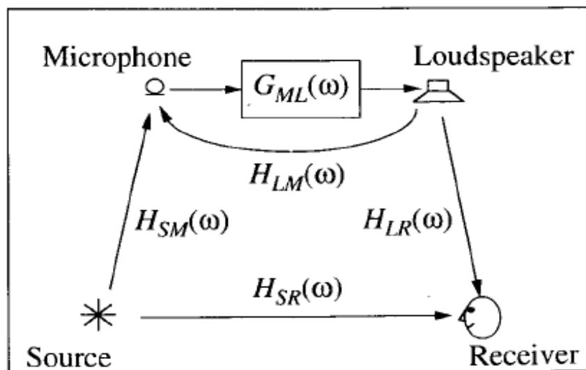
Figure 4.1: A basic model of an electro-acoustic system with the relevant transfer functions. Indices mean: S...source, R...receiver, M...microphones, L...loudspeakers. [Svensson, 1995]
