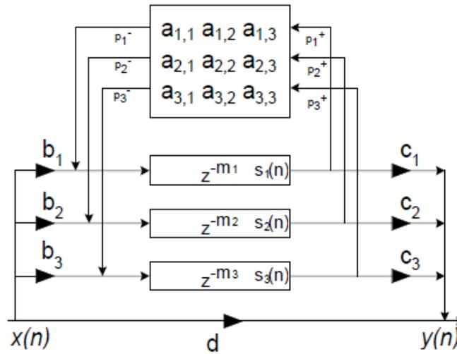
Figure 4.13: Feedback Delay Network of 3rd order. [Gardner, 1997]
