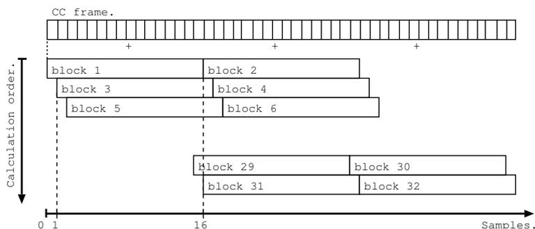
Figure 4.7: Merging algorithm for the linewise decomposition.
