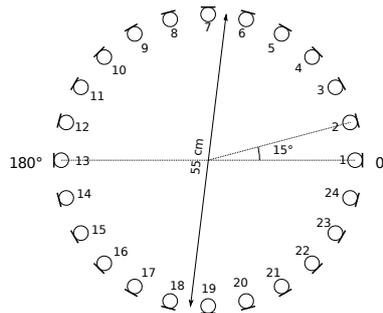
Figure 2.2: Scheme of the microphone array.
