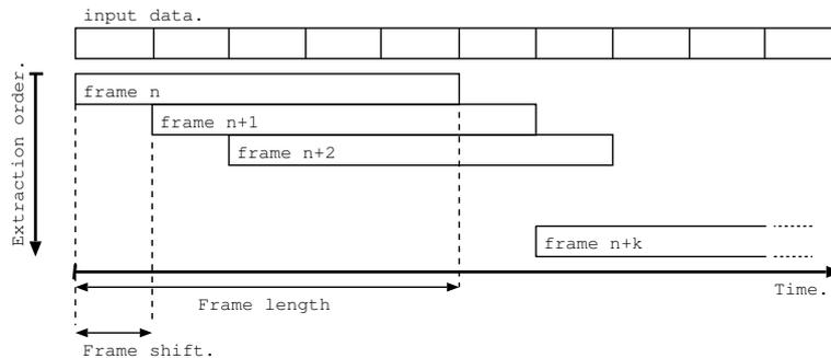
Figure 3.1: The frame mechanism.
