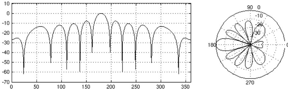
Figure 5.4: Directivity pattern of the circular array for an input frequency  $f = 1500\text{Hz}$  and  $\theta_s = 180^\circ$ .
