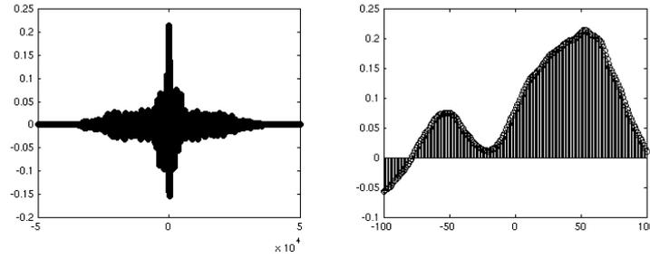
Figure 2.4: Cross correlation between  $m_1$  and  $m_{13}$ . Analysis time  $\approx 1s$ , sampling frequency = 48kHz.
