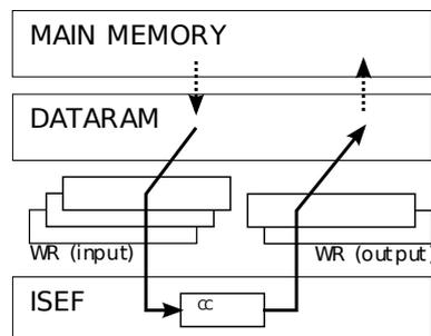
Figure 4.8: Data flow in the case of WRs use.
