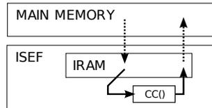
Figure 4.9: Data flow in the case of IRAM use.
