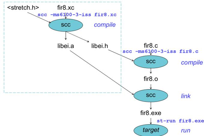
Figure 1.3: Building Process of an ISEF configuration.
