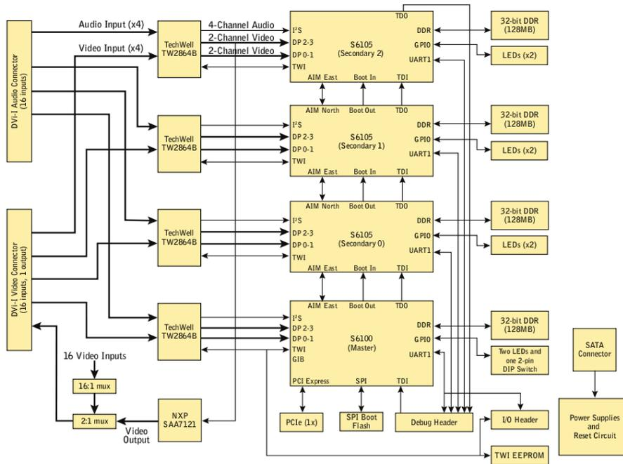
Figure B.3: VRC6016 board block diagram.
