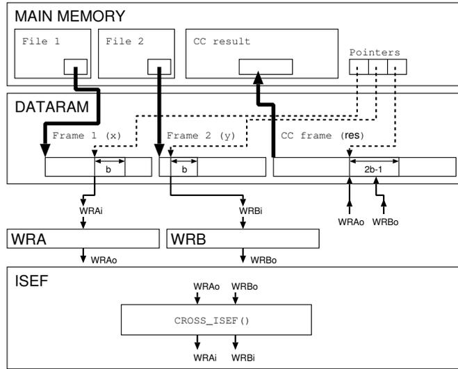
Figure B.7: Data flow in the case of ISEF use with square decomposition.
