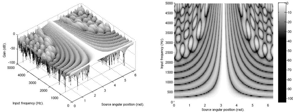
Figure 5.5: Effect of input frequency on directivity pattern,  $\theta_s = 180^\circ$ .
