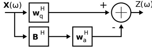
Figure 5.7: Mathematical description of the GSC beamformer.
