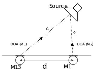
Figure 2.5: Simple case of near field configuration.
