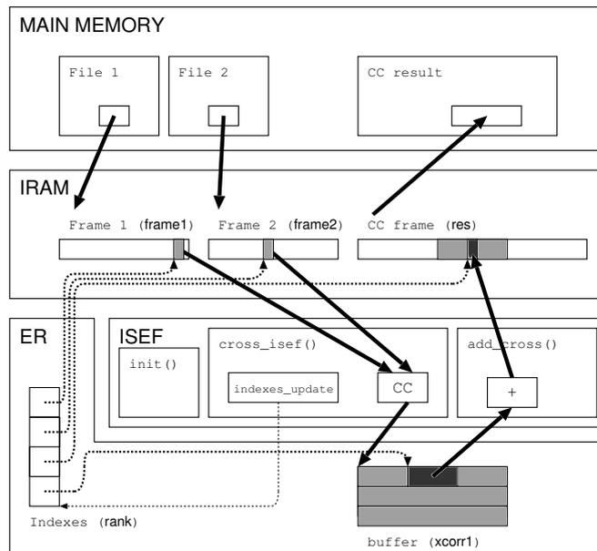
Figure B.10: Data flow in the case of IRAM use.
