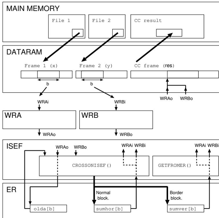
Figure B.8: Data flow in the case of ISEF use with diagonal decomposition.
