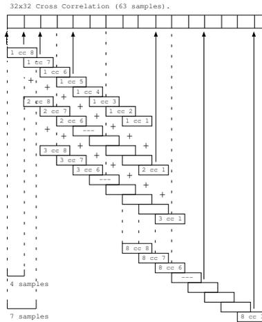
Figure 4.3: Principle of the merging algorithm for square decomposition.
