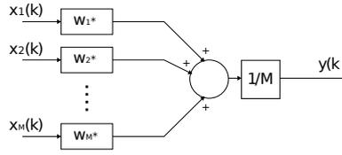
Figure 5.3: The delay and sum beamformer.
