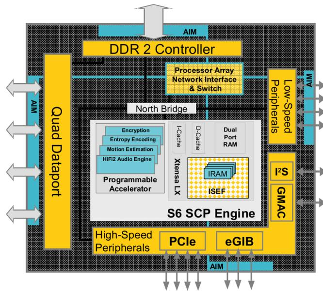
Figure B.4: Architecture of the Xtensa processor.
