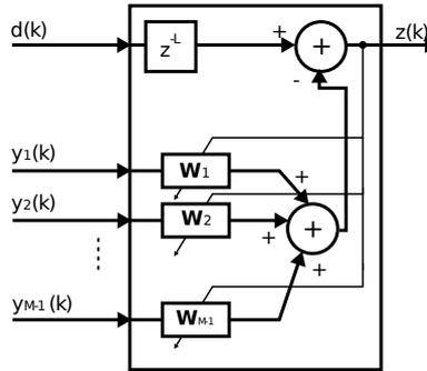
Figure 5.8: Multiple input canceler for the NLMS algorithm.
