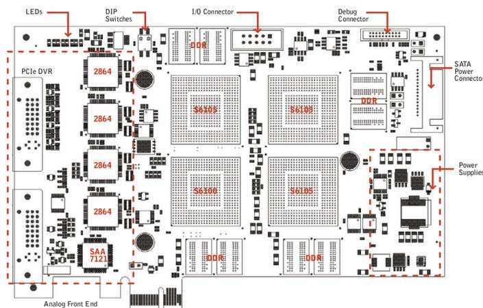
Figure B.2: VRC6016 board layout.
