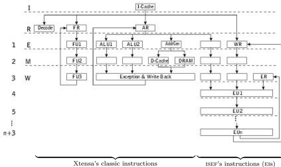
Figure 1.2: The extended pipeline structure.
