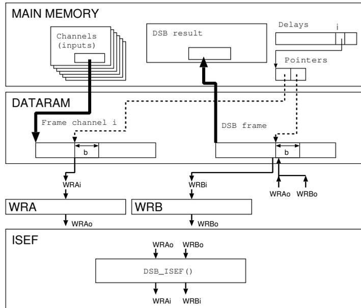
Figure B.14: Data flow of the DSB implementation.
