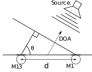
Figure 2.3: Simple case of source localization.
