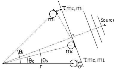
Figure 5.1: Highlighting of  $\tau_{m_c, m_i}$  under the far field assumption.
