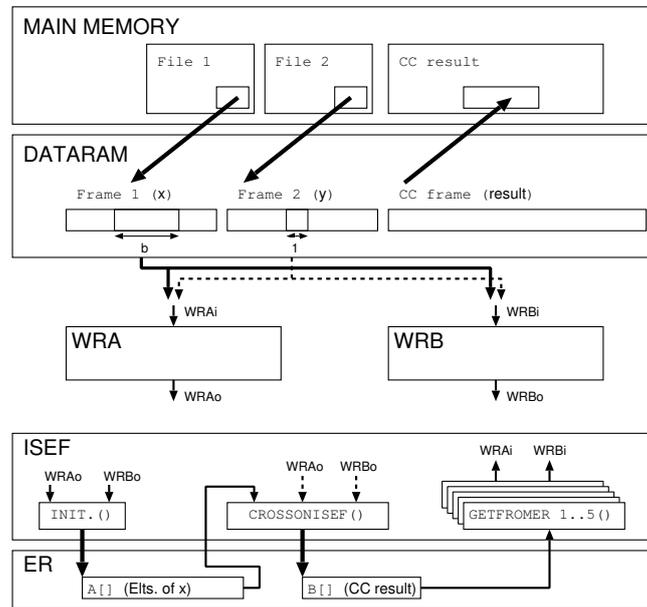
Figure B.9: Data flow in the case of ISEF use with linewise decomposition.
